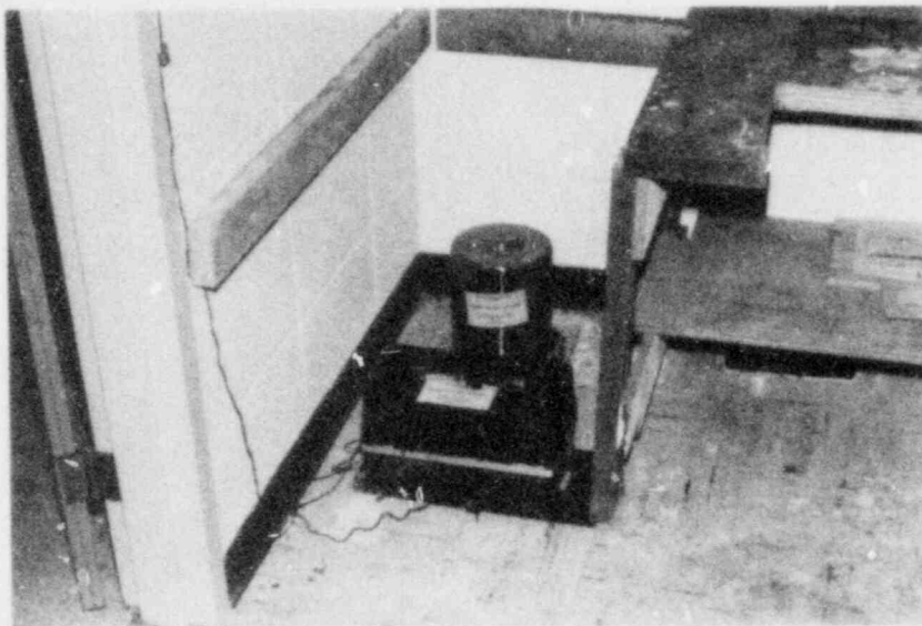
SMA-1 ACCELEROGRAPH GOULD HALL - BASEMENT VIEW: SOUTHWEST
