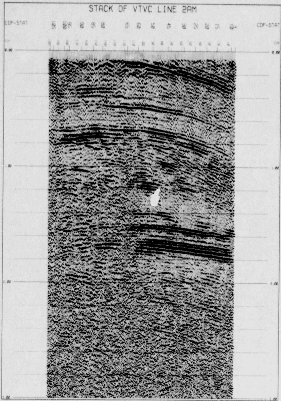
Figure 4. Stack (unmigrated) Line VTVC2A: Note improvement in reflection continuity and increase in spatial and temporal resolution over Figure 3. The dimensions of the plot are the same as Figure 3; however, the trace spacing is reduced from 35 m to 30 m. Filter: 6-10-80-85 Hz. Horizontal scale \approx 1'' = 1500 m. This figure is the same as Plate I.
