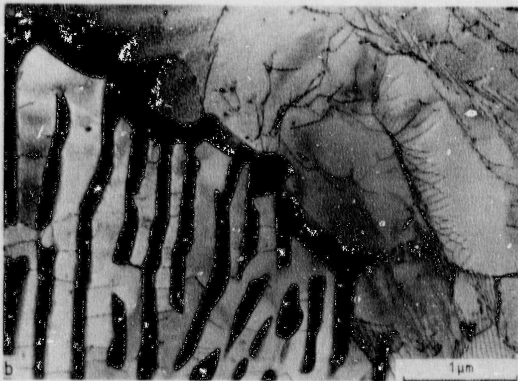
Fig. 7 Transmission electron microscopy microstructures of as-processed and cyclically prestrained A 516 Gr. 70 steel: (a) through (d) as received, unstrained; (e) through (h) 2% maximum strain (100 cycles); and (i) through (l) 20% maximum strain (25 cycles).
