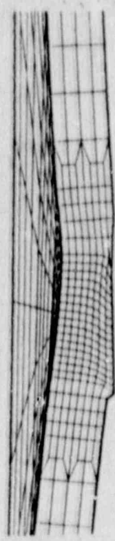
Figure 5.1.41 Side View of Deformed Shape of the Liner in the Stud-Shear Problem With Initial Membrane Tension (Analysis 1b)
