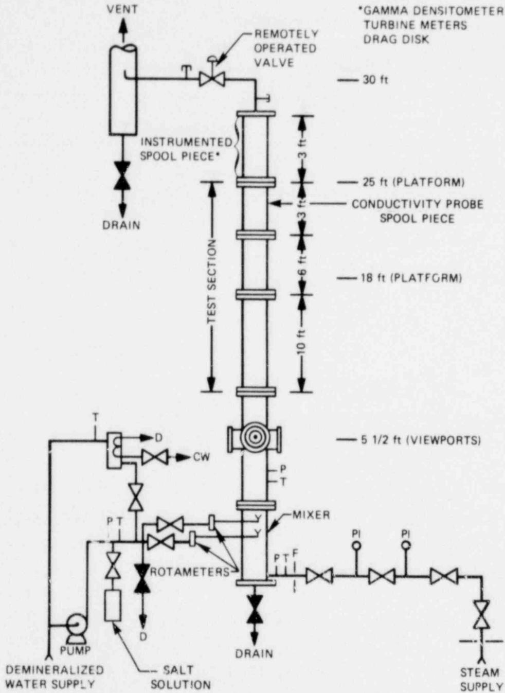
Fig. 19. AIRS steam-water test stand.
