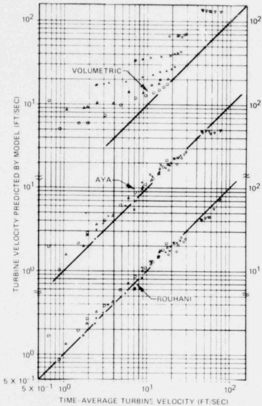
Fig. 10. Turbine velocity predicted by three turbine models vs actual mean turbine velocity recorded in horizontal flow. Solid lines denote perfect agreement for each model.
