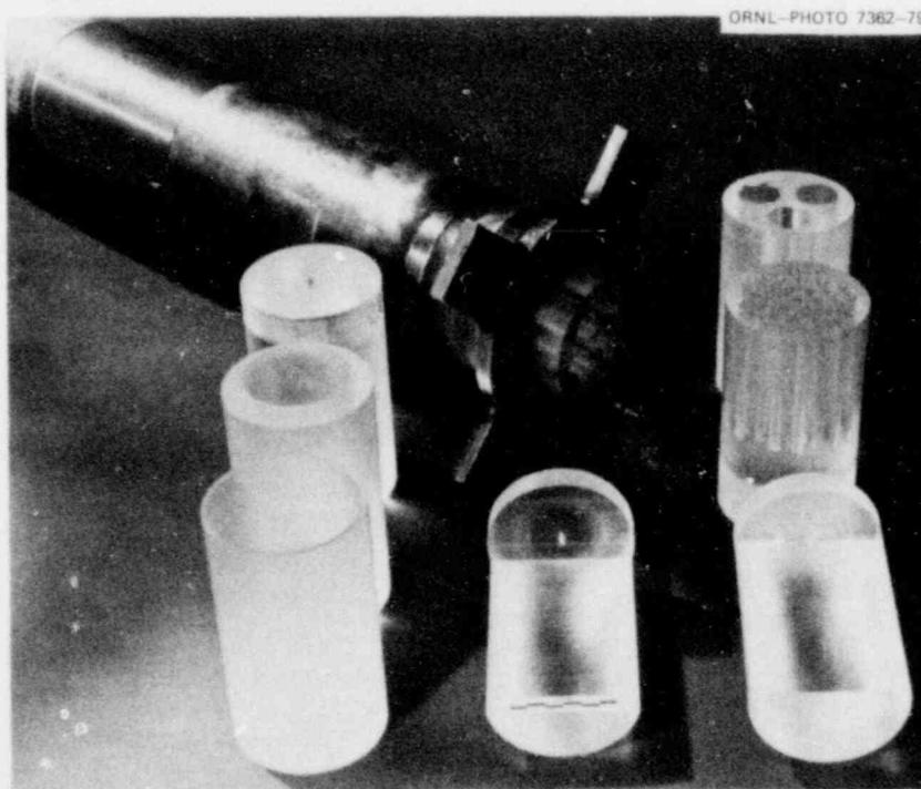
Fig. 8. Flexiglas inserts representing two-phase flow regimes, used to evaluate accuracy of densitometer measurements.
