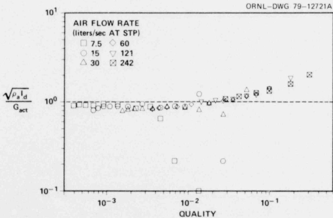
Fig. 16. Ratio of mass flux determined using densitometer and drag flowmeter to actual mass flux in horizontal two-phase flow.
