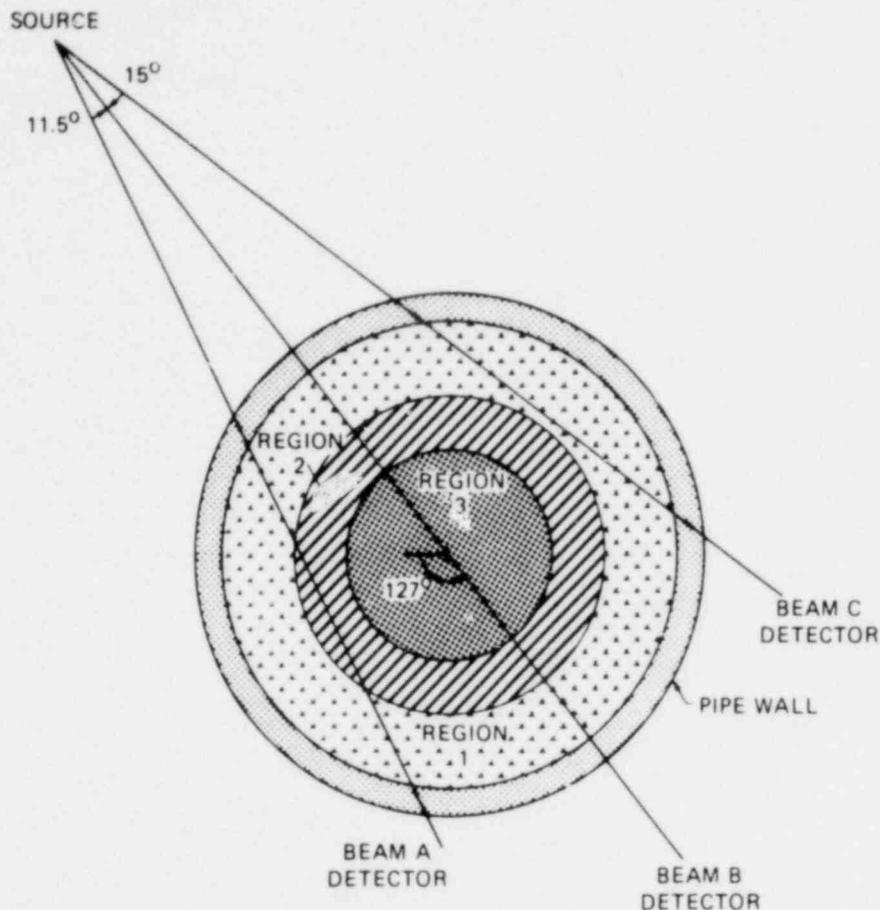
Fig. 6. Diagram showing uniform density regions used in annular model for reduction of three-beam densitometer data.
