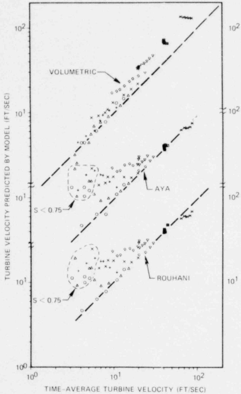
Fig. 11. Turbine velocity predicted by three turbine models vs actual mean turbine velocity recorded in vertical downflow. Solid lines denote perfect agreement for each model.
