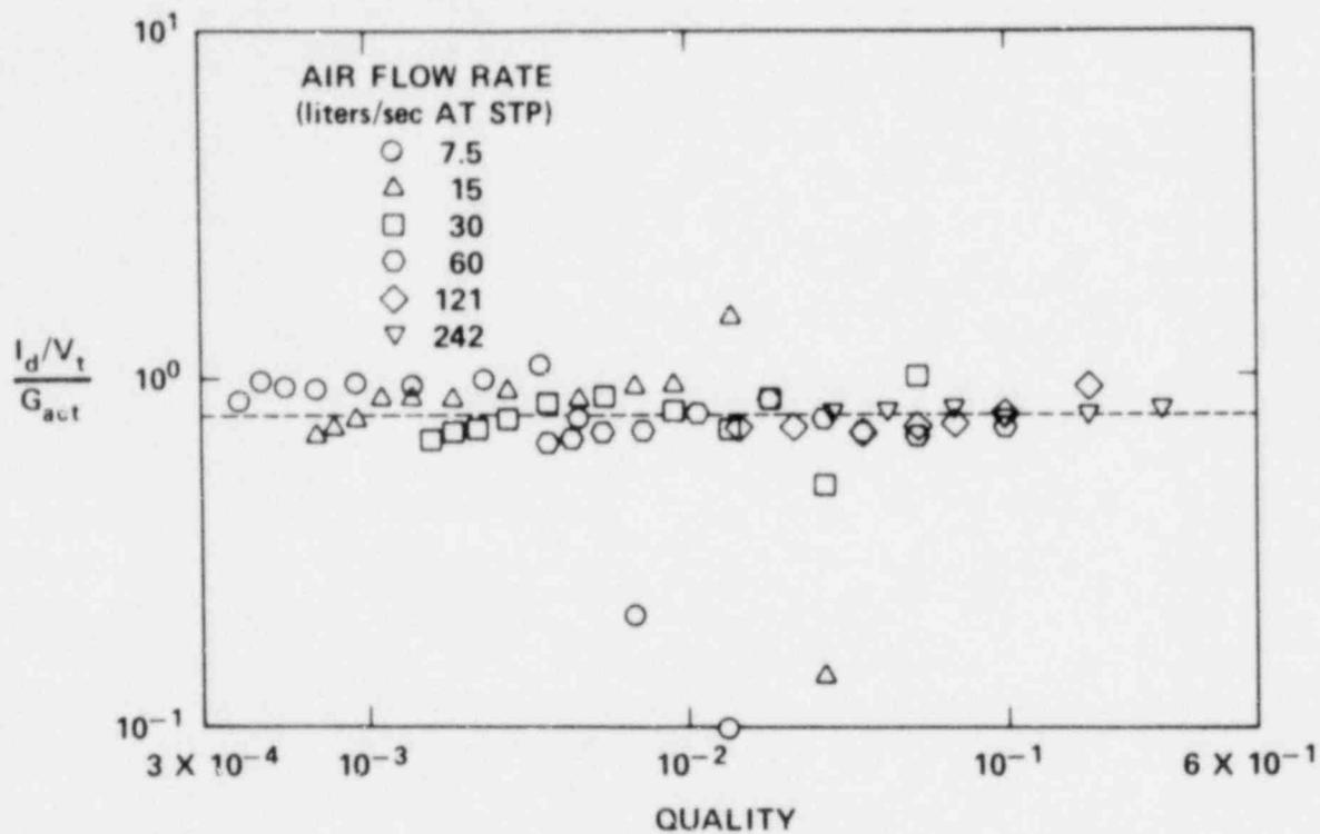
Fig. 17. Ratio of mass flux determined using turbine and drag flowmeter to actual mass flux in horizontal two-phase flow.
