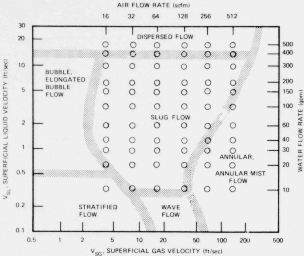
Fig. 3. Flow pattern map proposed by Mandhane et al. for horizontal flow with locations of data points used in air-water studies.
