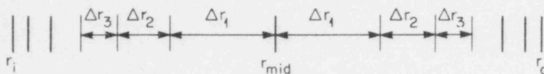
Fig. 2. Mesh Spacing Scheme Used in Material Zone.
