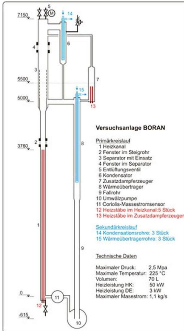
Figure BV-1. BORAN Schematic
