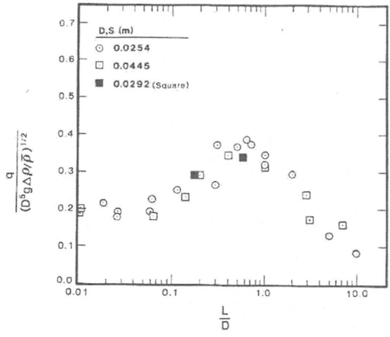
Figure V-5. Purging/Flooding Flow, Reproduced from Figure 4 of Reference [17]
