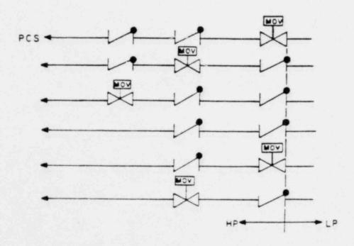
Figure 1. Valve Configurations Designated by NRC to be Included in This Technical Evaluation
