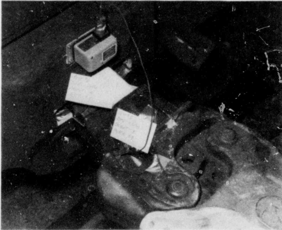
Figure 5. Coupler Force and Displacement Instrumentation at Struck End of Car - Tests 1-5
