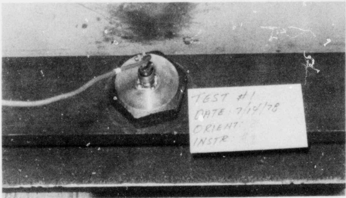
Figure 4. Vertical Tiedown Bolt at Near Middle of One Side of Hallum Cask Skid - Test 1
