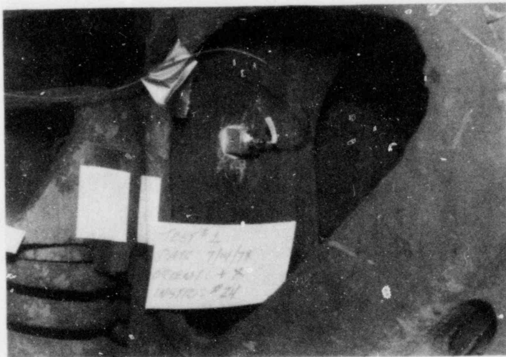
Figure 16. Accelerometer Placement on Rail Truck Structure at Far End of Car - Tests 1-5
