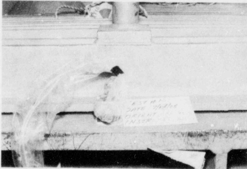
Figure 28. Accelerometer Placement on Top of Scrap Cask at Struck End of Car - Tests 10 and 11
