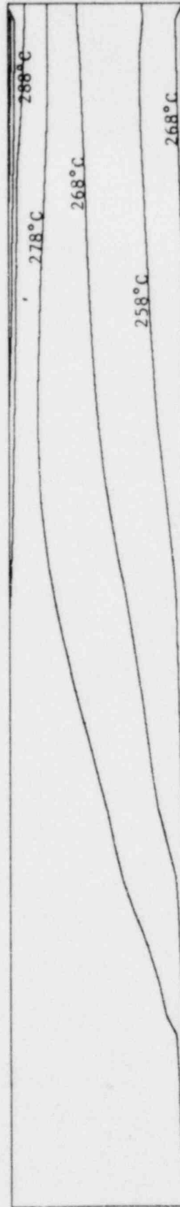
Fig. 12. Temperature Distribution of Vertical Cross Section through Centerline at t = 200.0 sec.
