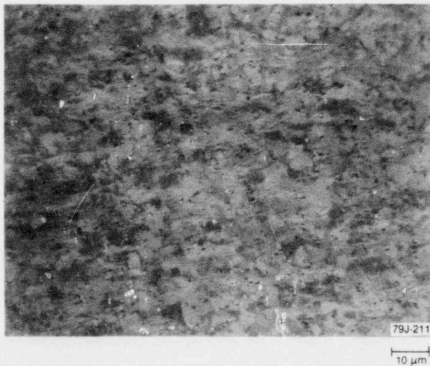
Figure 61. Rod 312-4 transverse cladding microstructure (Sample M4-3) from 0.53 to 0.55 m.
