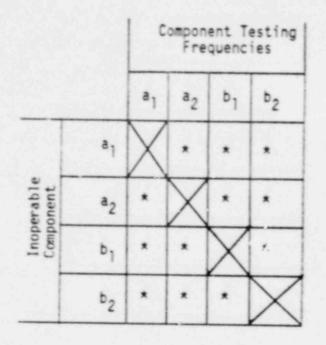
Key: \*Within 4 hours and every 12 hours thereafter a<sub>1</sub> Offsite power circuit No. 1 a<sub>2</sub> Offsite power circuit No. 2 b<sub>1</sub> Class 1E diesel generator (Red) b<sub>2</sub> Class 1E diesel generator (Green)
