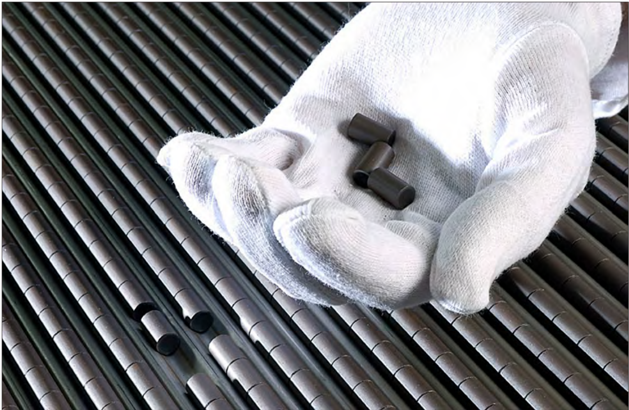
Nuclear fuel pellets are stacked vertically in long metal tubes to power commercial nuclear reactors. There are many steps involved in processing uranium before it is fabricated into nuclear fuel. Courtesy of Areva.
