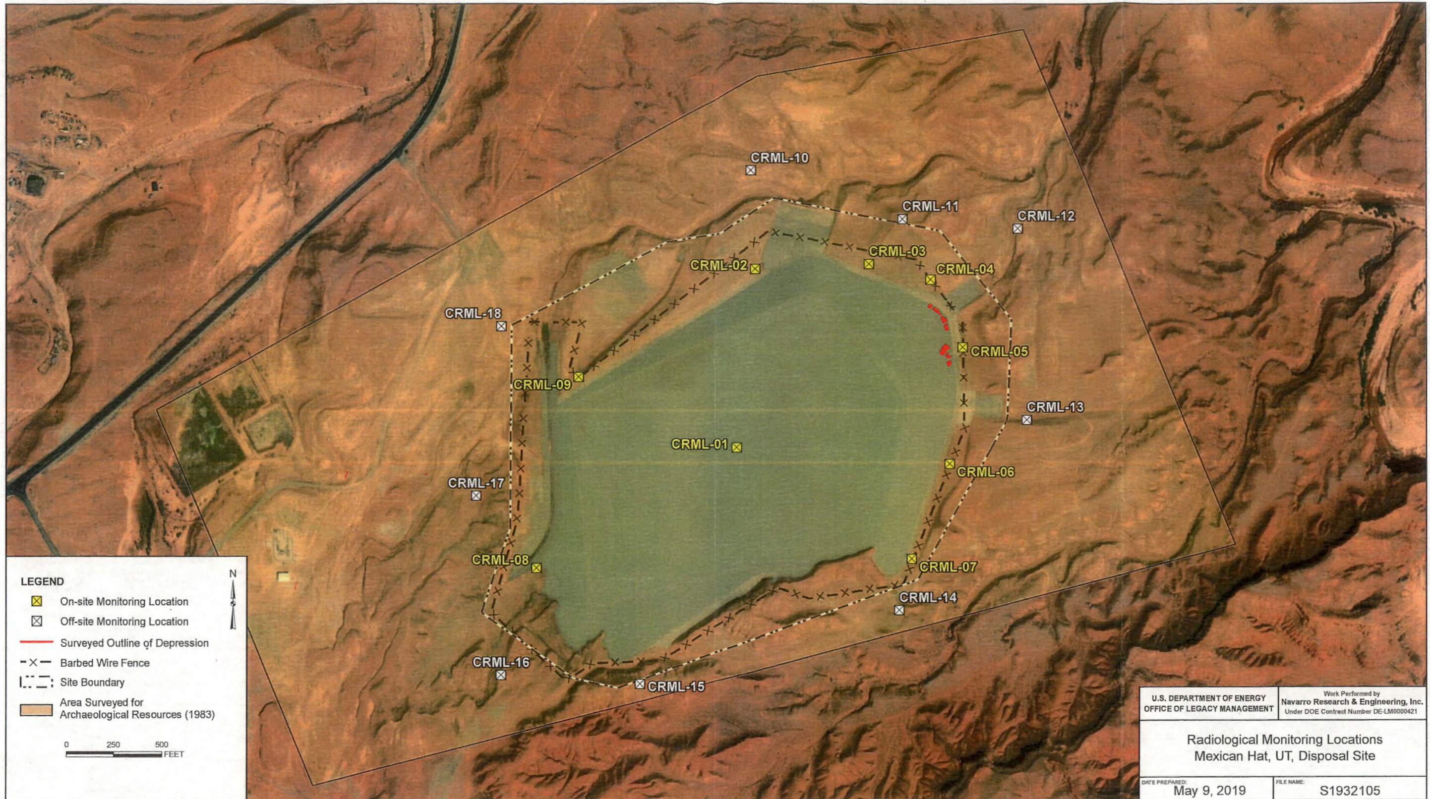
Figure 2. Radon Detector and TLD Placement Locations at the Mexican Hat, Utah, Disposal Site
