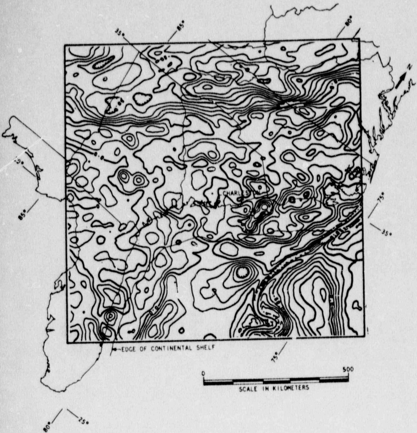
Figure 6-5. Contour plot of Bouguer Gravity Anomalies. Contour interval is 10 milligals.
