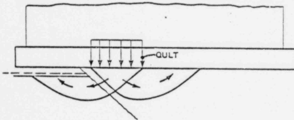
RAPID LOADING AT QULT  $\approx$  20 ksf CAUSES LOCAL FAILURE OF FOUNDATION SOILS
