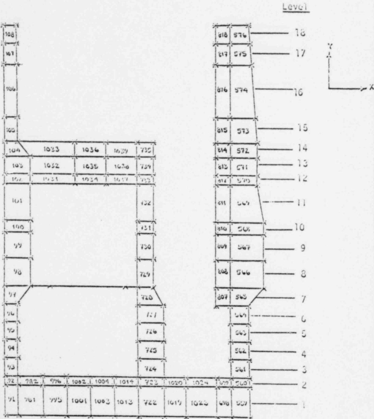
FIGURE A-1 VERTICAL SECTION OF REACTOR BUILDING CORE MODEL
