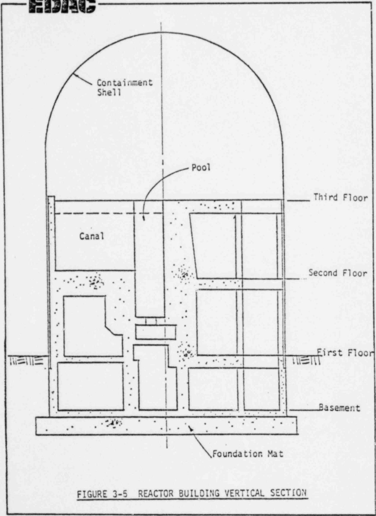
FIGURE 3-5 REACTOR BUILDING VERTICAL SECTION
