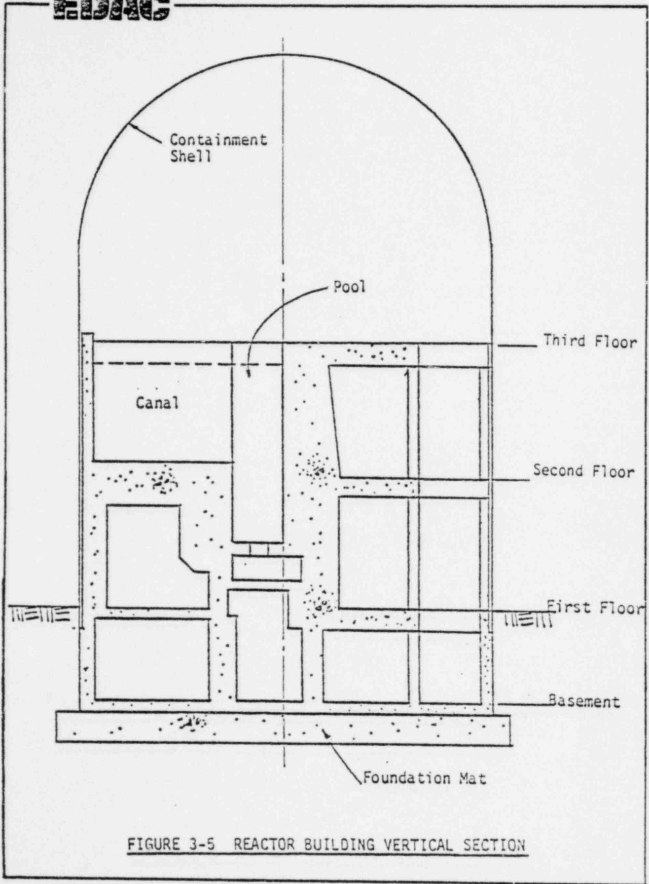
FIGURE 3-5 REACTOR BUILDING VERTICAL SECTION
