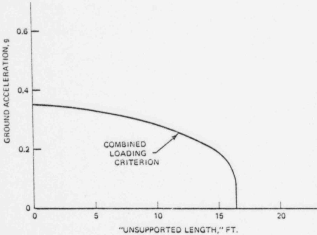
FIGURE 2 COMBINATION OF LOADINGS BASED ON PROBABILISTIC CONSIDERATIONS (AFTER REF. 3)
