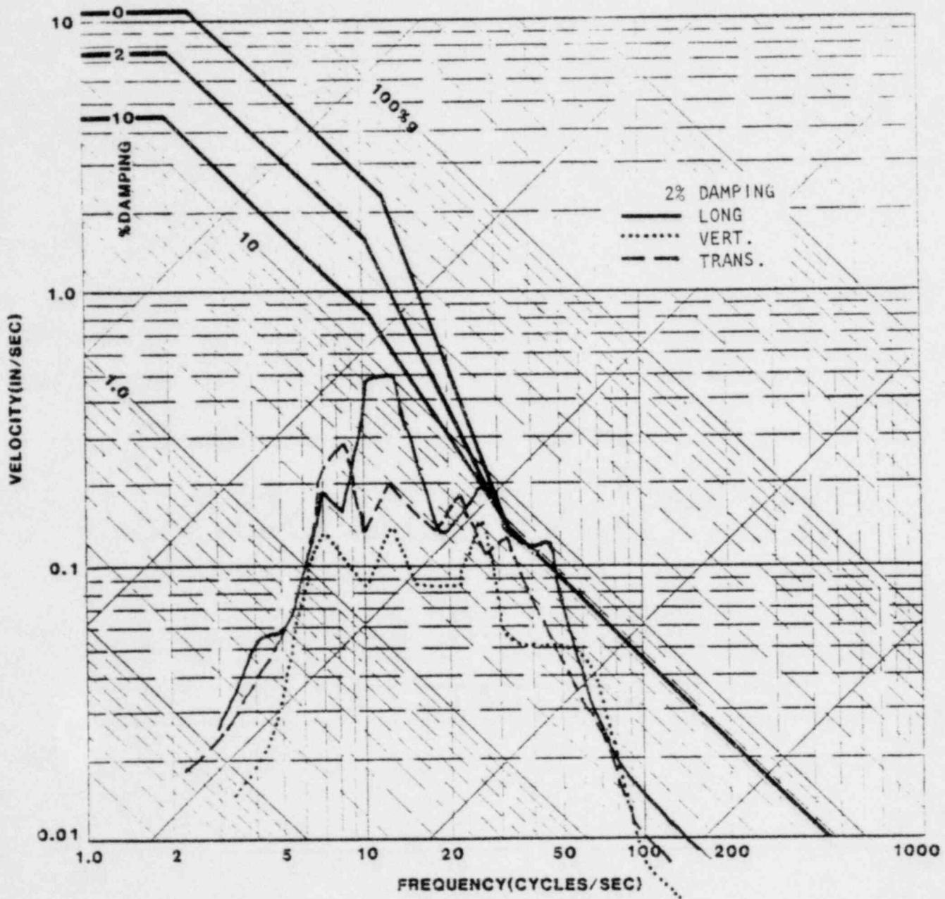
UBE DESIGN SPECTRA AND 2% SPECTRA OF BLAST OF 2/4/80 (410LBS)
