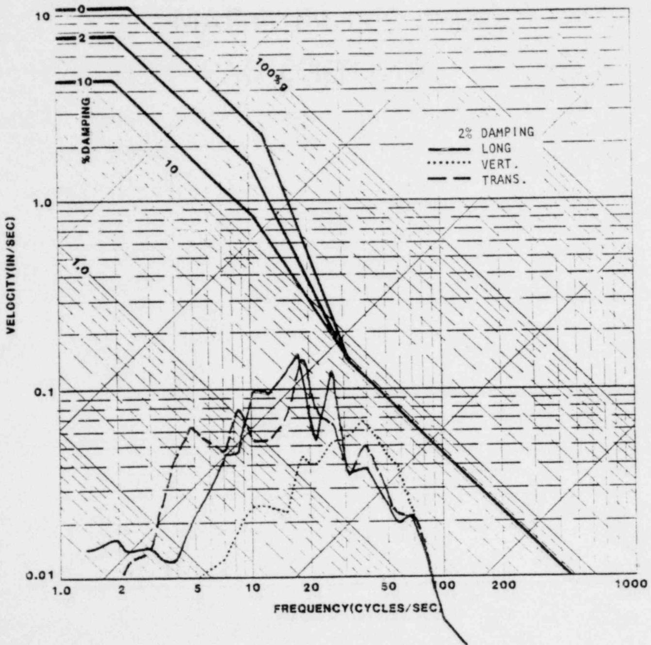
OBE DESIGN SPECTRA AND 2% SPECTRA OF BLAST OF 2/4/80 (410 LBS.,
