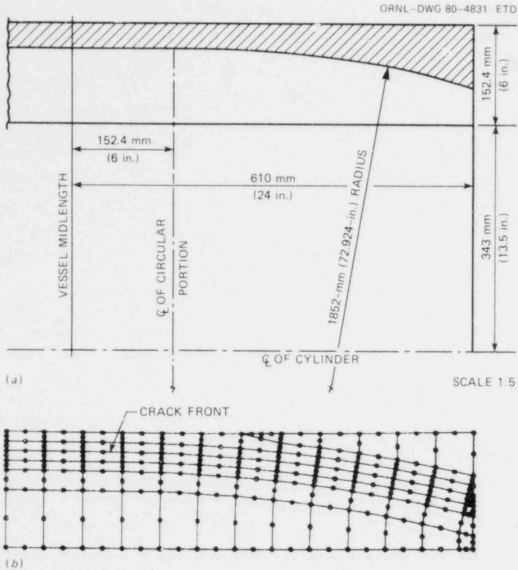
Fig. 4.4. Idealization of final arrested crack front of TSE-5 for purposes of 3-D FE analysis. (a) Partial longitudinal section through vessel wall. (b) FE model of cylinder wall used to generate 3-D mesh by rotating it about cylinder axis.
