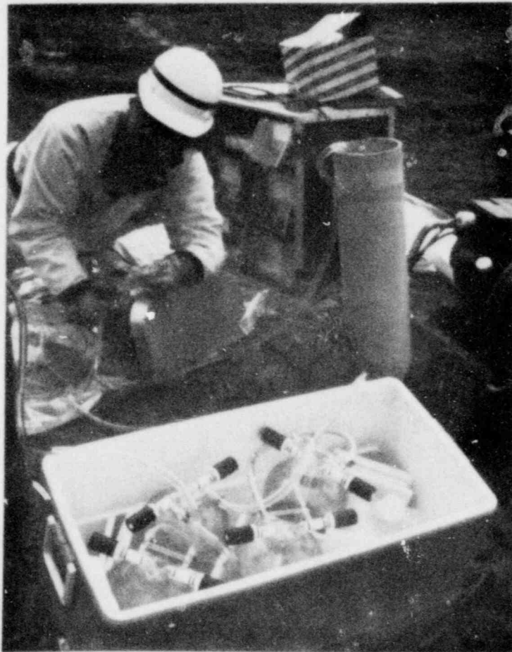
Figure 5.3. Portable anoxic collection system used to sample trench water from low-level radioactive waste disposal sites.
