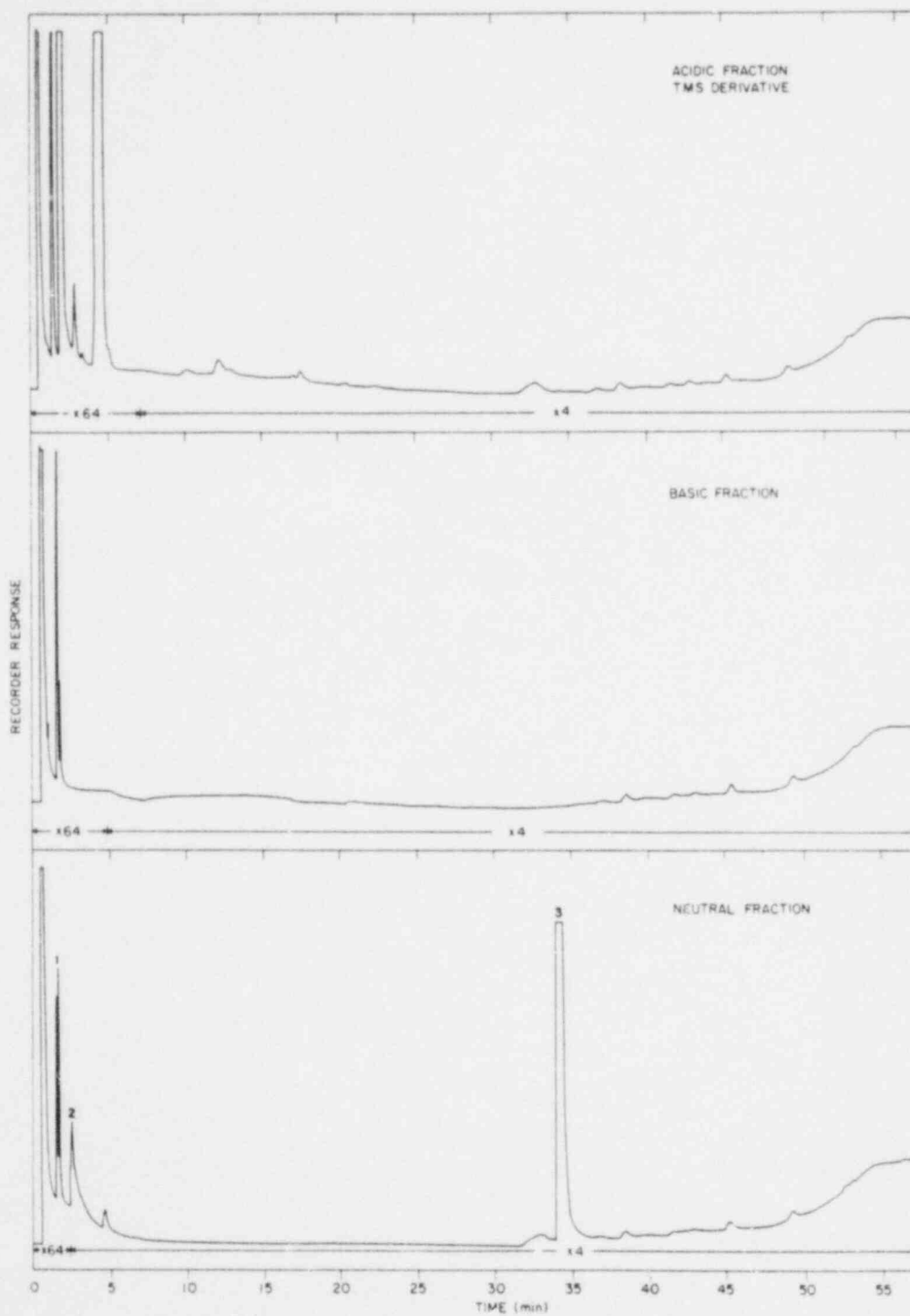
Figure 5.12. Gas chromatogram of methylene chloride extract of trench 33L-18 water sample from Maxcy Flats, Kentucky, disposal site.
