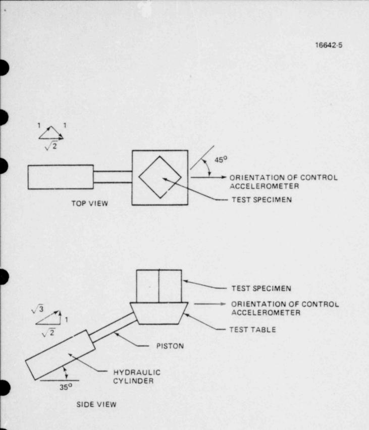
Figure 2 Test Specimen Orientation
