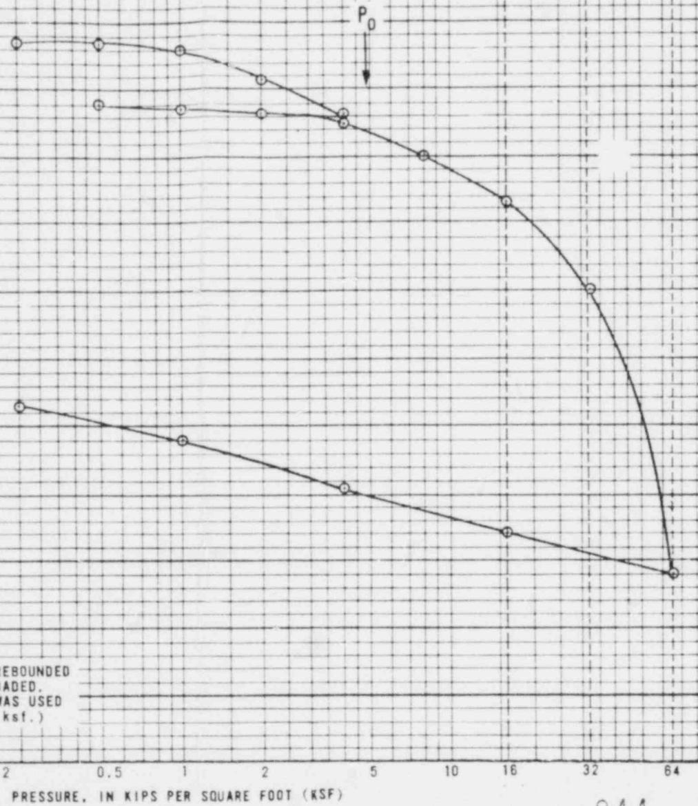
NOTE: SAMPLE WAS SUBMERGED AT 1.0 ksf, REBOUNDED TO 0.5 ksf FROM 4.0 ksf, THEN RELOADED. (A STRESS-INCREMENT RATIO OF 1.0 WAS USED FOR ALL LOAD INCREASES UP TO 64.0 ksf.)
