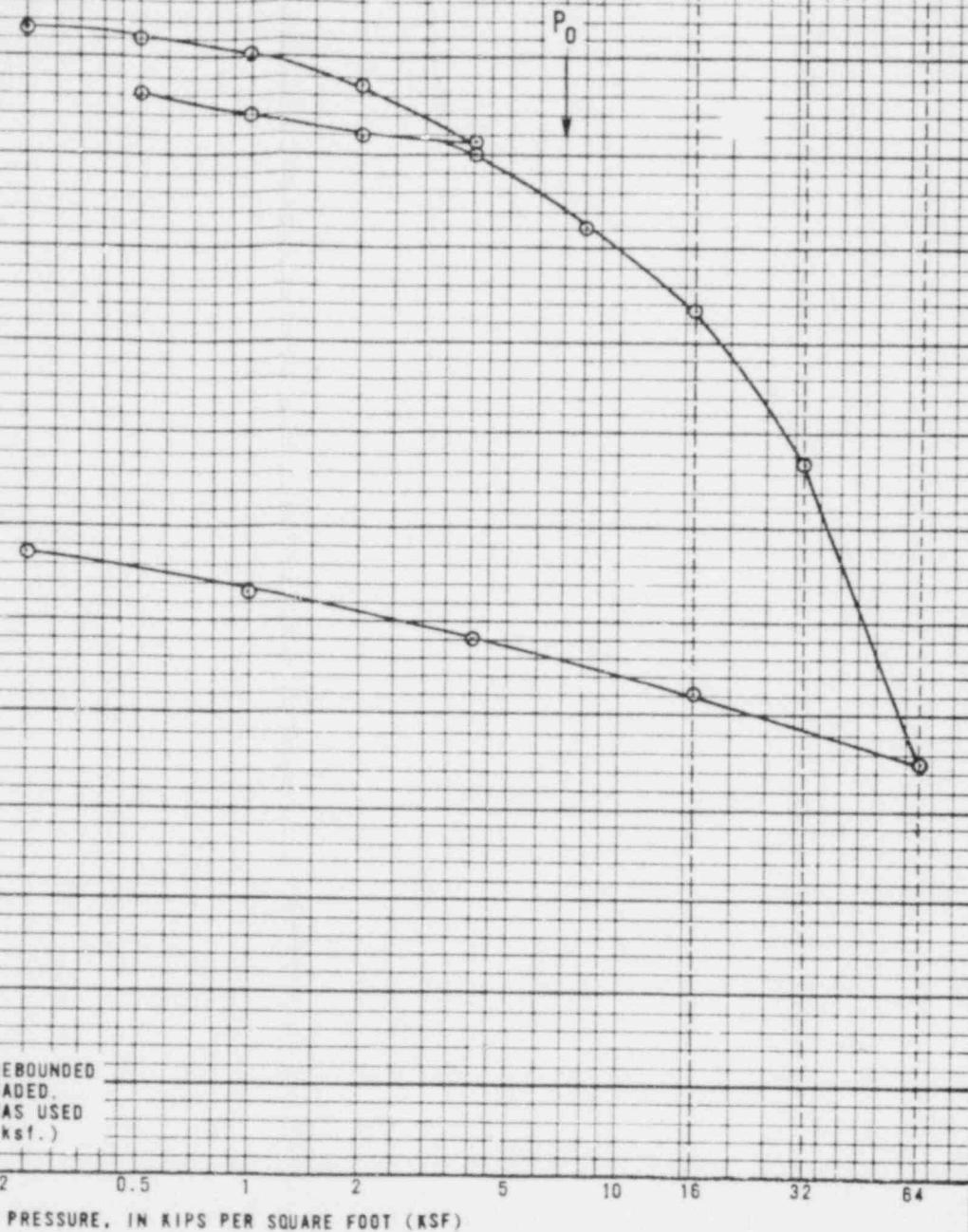
NOTE: SAMPLE WAS SUBMERGED AT 1.0 ksf, REBOUNDED TO 0.5 ksf FROM 4.0 ksf, THEN RELOADED. (A STRESS-INCREMENT RATIO OF 1.0 WAS USED FOR ALL LOAD INCREASES UP TO 64.0 ksf.)
