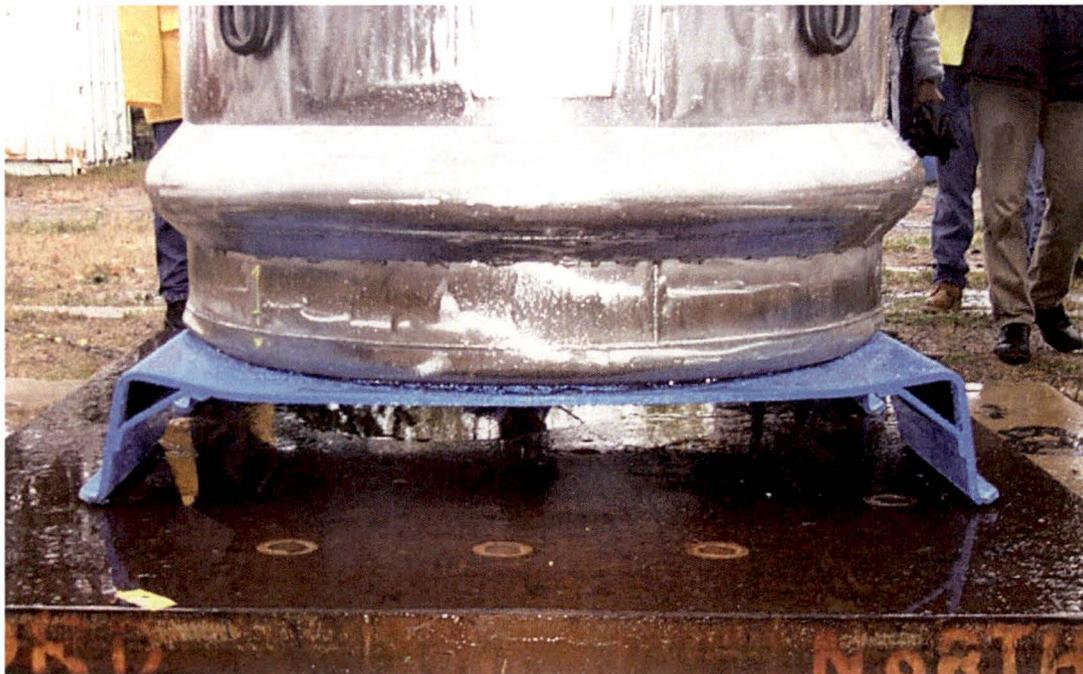
**Figure 12, Damage after 1.2m normal drop.**
