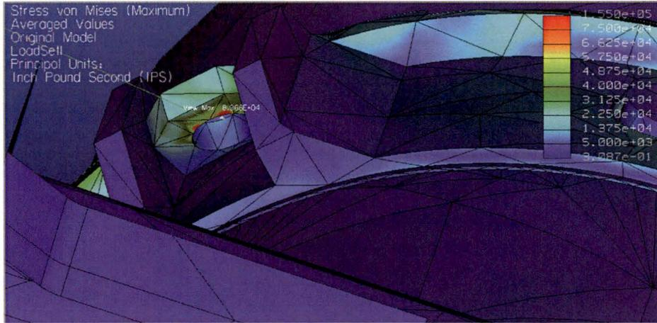
Figure A2.10.2-4: Stresses in the Tie-Down Lug
