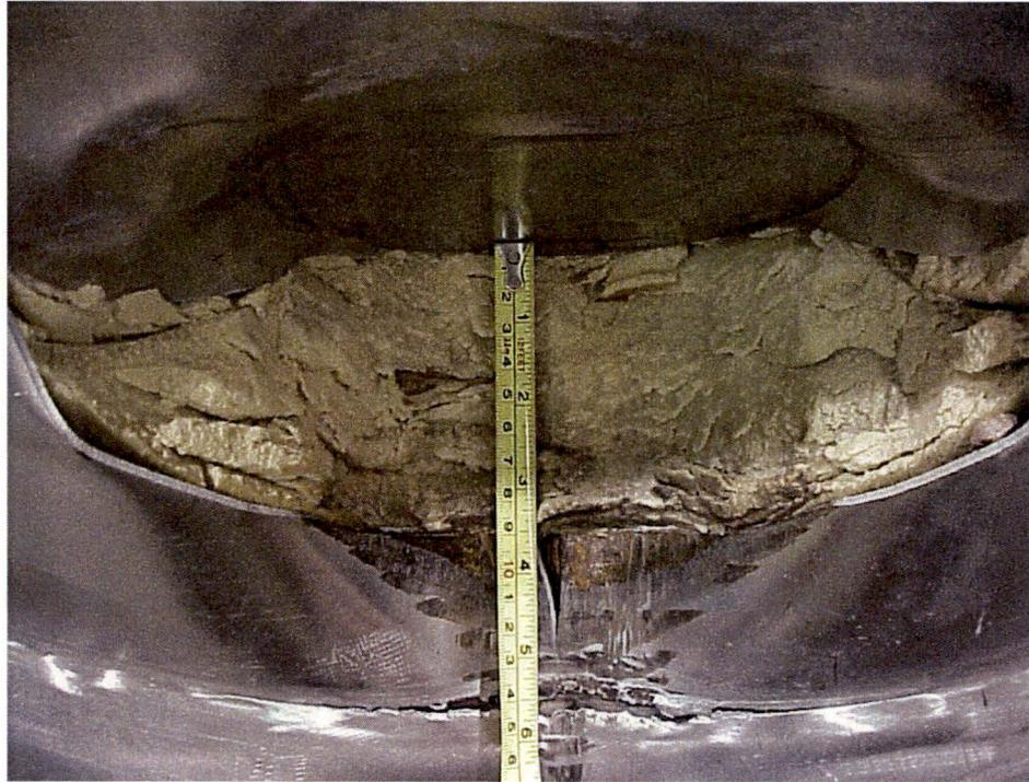
**Figure 20, Detail of Skin Damage after Oblique Pin Drop**
