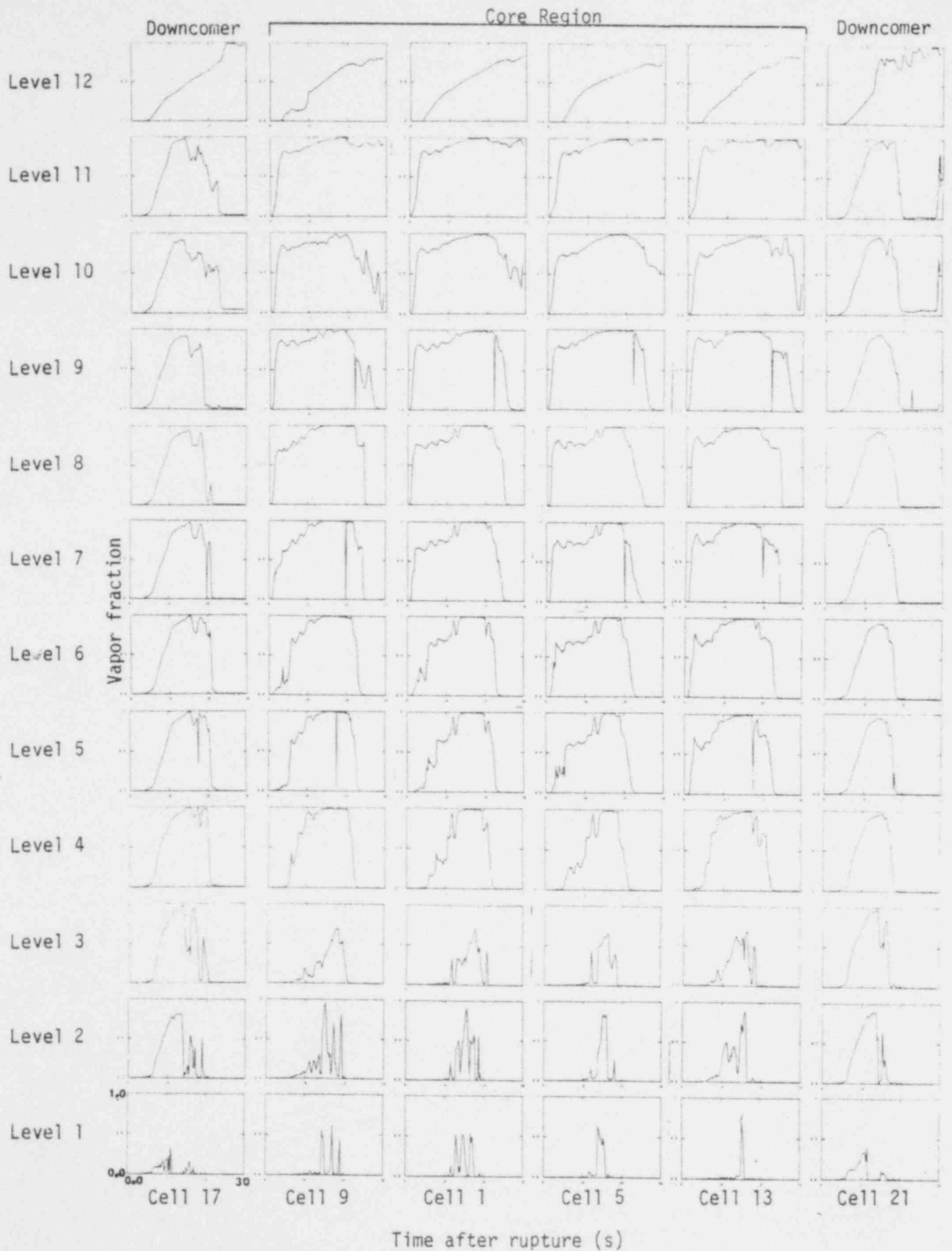
Figure 22. Vapor fraction of vessel theta section cutting through the broken broken loop cold leg connection.
