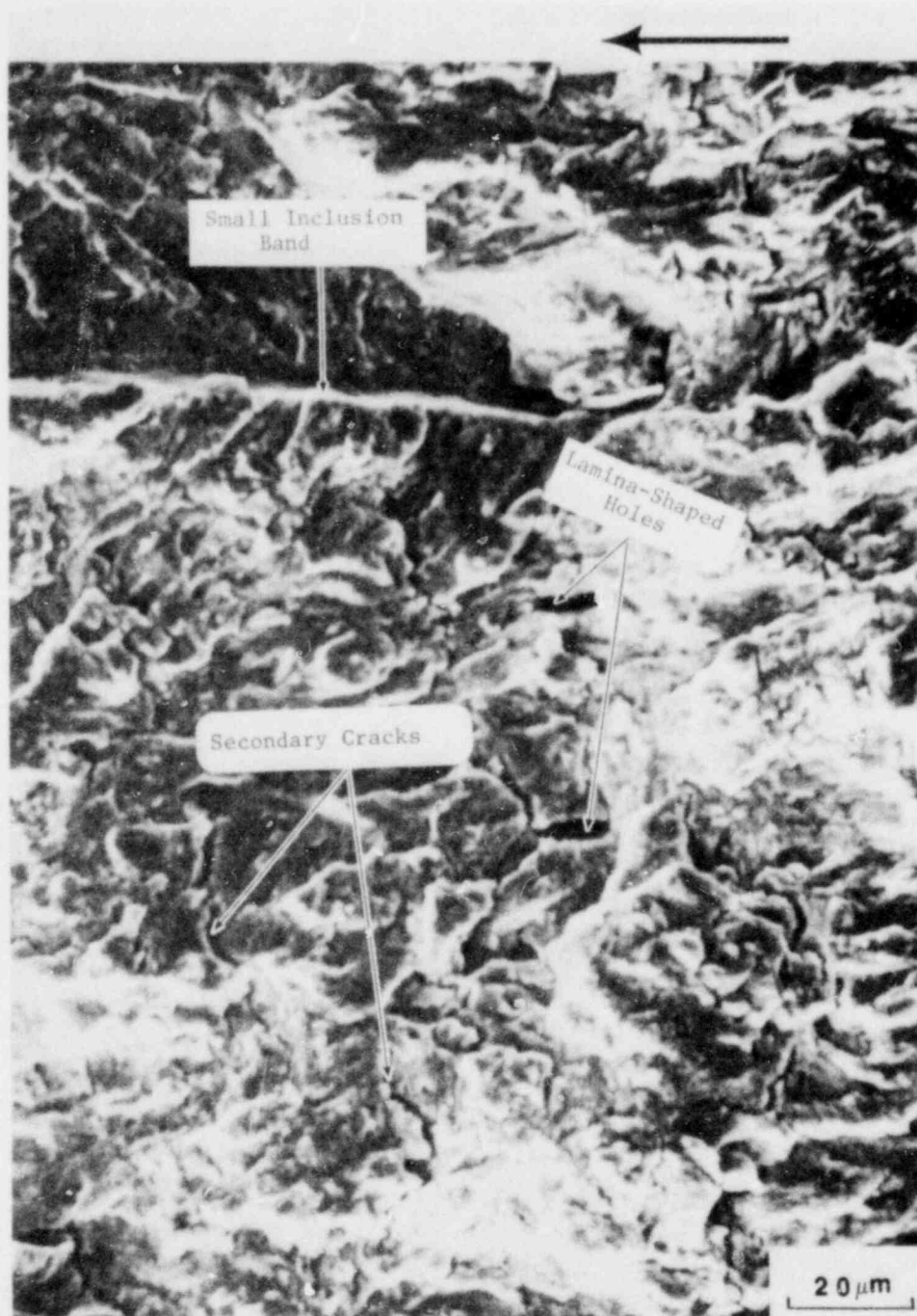
Fig. 34 Fracture surface of A302-B ferritic steel specimen cut along L-T direction (VADA2) tested in air at room temperature. Arrow shows direction of macroscopic crack propagation. SEM micrograph shows small inclusions and lamina-shaped holes present in the fracture surface. The lamina-shaped holes are believed to represent the inclusion bands that are oriented perpendicular to main crack plane.
