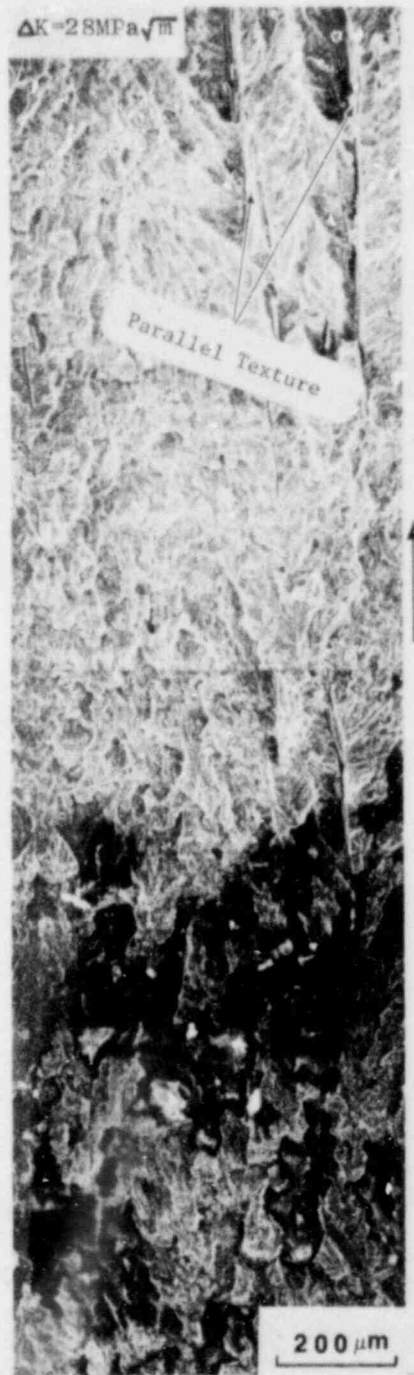
Fig. 32 Fracture surface of A302-B ferritic steel specimen cut along T-L direction (VABI), tested in air at room temperature with the lower starting \Delta K value. Arrow shows direction of macroscopic crack propagation. Series of SEM micrographs show transition region corresponding to 25 to 30 \text{MPa}\sqrt{\text{m}} \Delta K value, where inclusion bands begin to appear in fracture surface.
