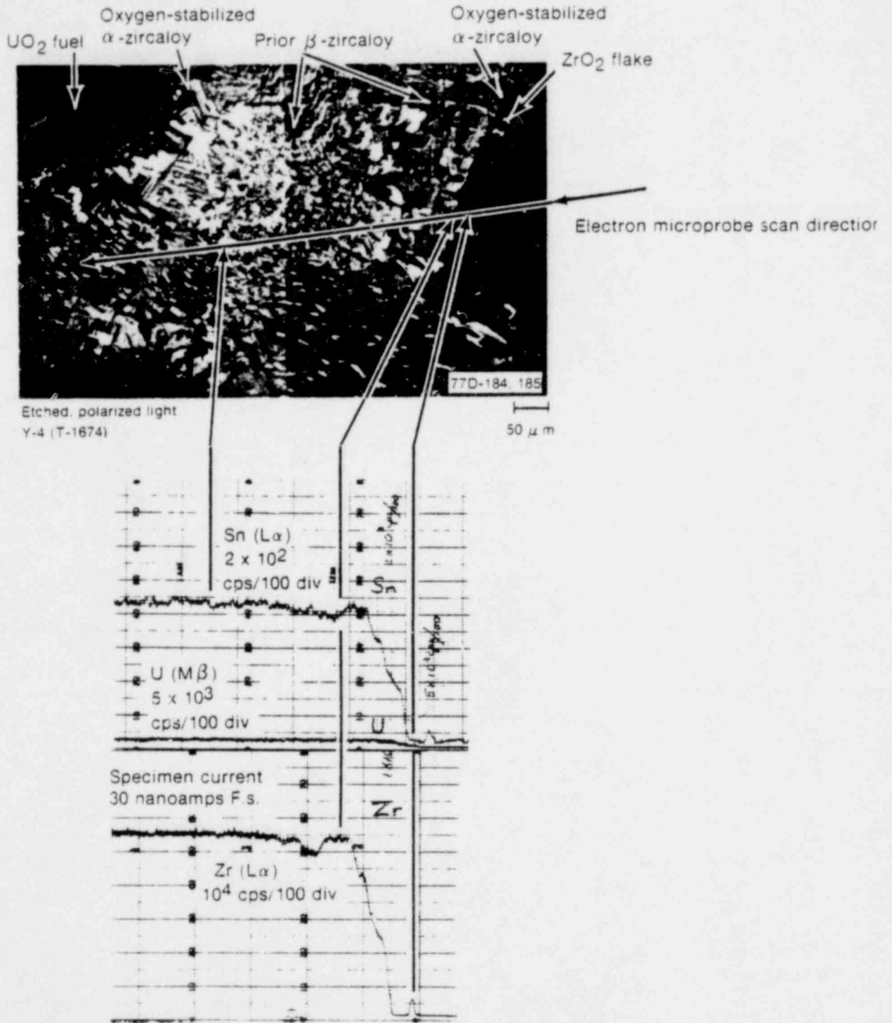
Fig. 51 Electron microprobe scan across the surface oxide and zircaloy cladding of Rod UTA-0014.
