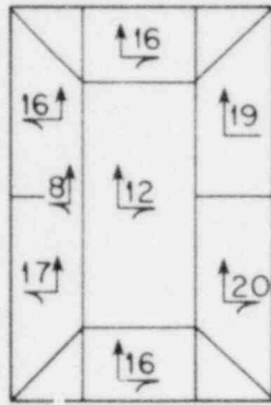
1st LAYER, 3/32-in. diam ELECTRODES
