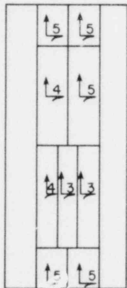
3rd LAYER, 1/8-in. diam ELECTRODES
