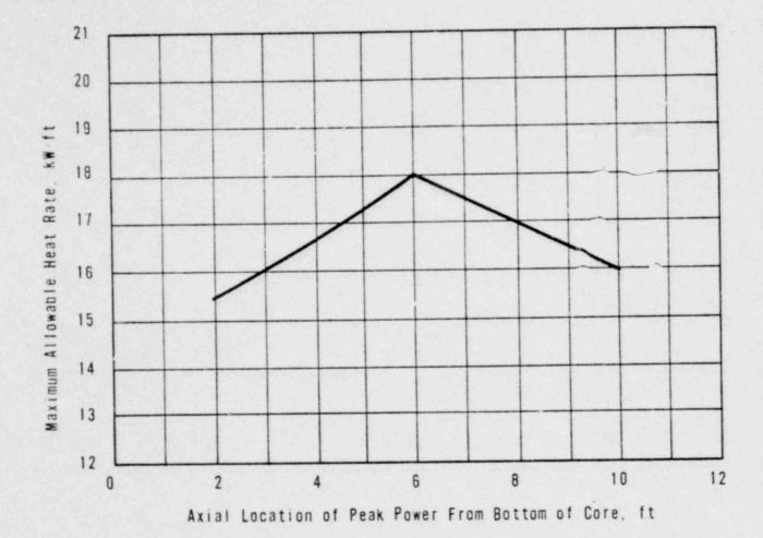
LOCA LIMITED MAXIMUM ALLOWABLE LINEAR HEAT RATE Figure 3.5.2-4
