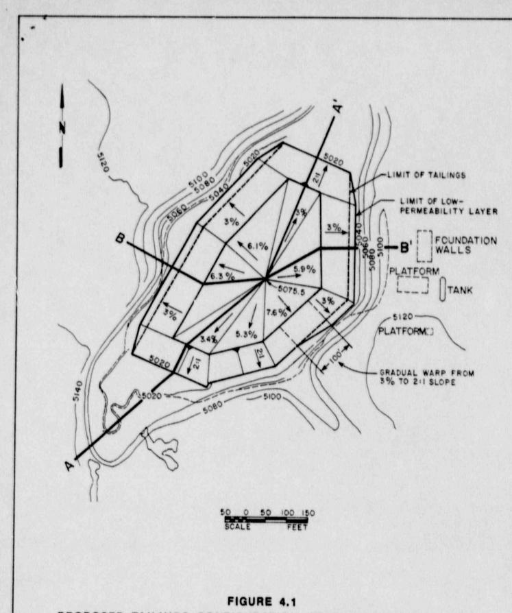
PROPOSED TAILINGS CONFIGURATION, STABILIZATION IN PLACE SPOOK SITE CONVERSE COUNTY, WYOMING
