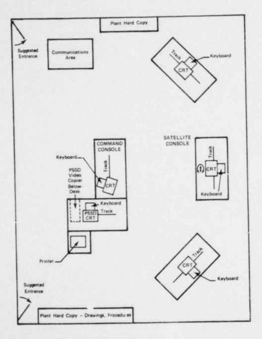
Figure 2-1. Typical Onsite Technical Support Center Facility Layout
