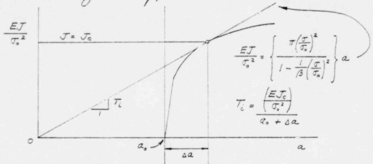
$$T_i = \frac{\pi \left( \frac{\sigma}{\sigma_0} \right)^2}{1 - \frac{1}{3} \left( \frac{\sigma}{\sigma_0} \right)^2} \quad \left( \frac{\sigma}{\sigma_0} \right)^2 \left[ \pi + \frac{T_i}{\beta} \right] = T_i$$
