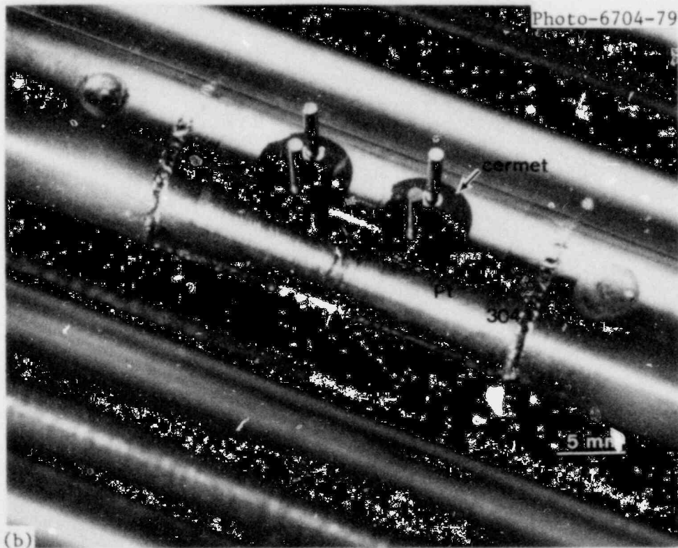
Fig. 31. Sensors on Instrumented Guide Tube Rods Shown Before 175°C (350°F) Steam-Water Tests at ORNL. (a) Flag-type probe on rod IF48-5. (b) Prong probe on level 7 of rod IP67-13.
