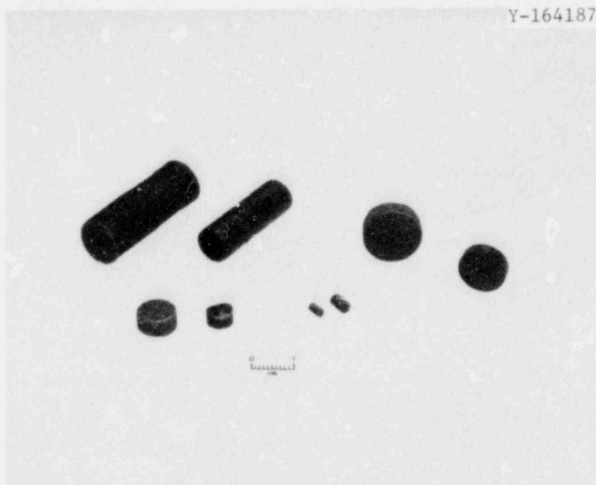
Fig. 6. Hot-Pressed Blanks of Platinized Alumina Cermet Both Before and After Grinding into Insulator Parts.
