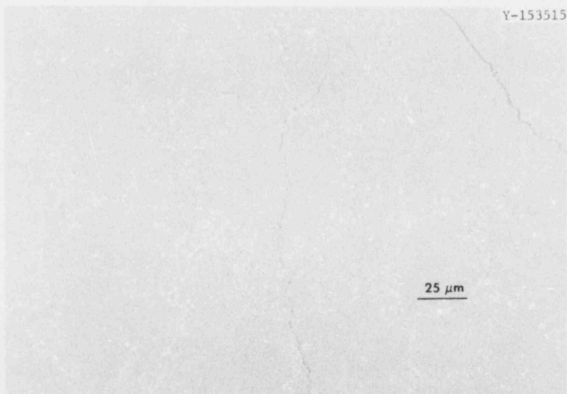
Fig. 5. Platinized Alumina Cermet Insulator After 20 Quenches from 520°C (970°F) Air into Water at 80°C (175°F). Although the structure contains some microcracks, they typically do not interconnect (after this many thermal shocks) to form a major leak path.
