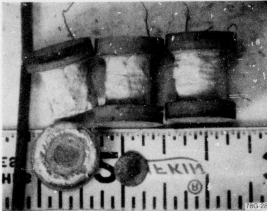
Figure G-5. Irradiated coils prepared on ceramic forms using Alloy 406 wire and Dylon C-7 cements.
