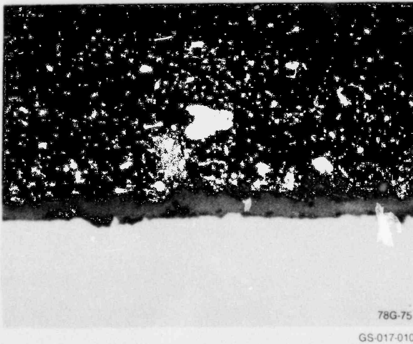
Figure F-14. Interface of 304 stainless steel disc with Dylon C-7 after irradiation (200X).
