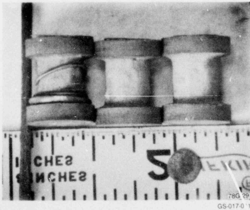
Figure G 2. Irradiated coils prepared on ceramic forms using Alloy 406 wire and Denex No. 2 cement. Three flux monitors are shown on one of the coils.
