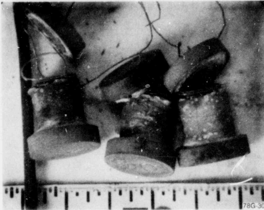
Figure G-1. Irradiated coils prepared on ceramic forms using Alloy 406 wire and Yellow Cerro cement.
