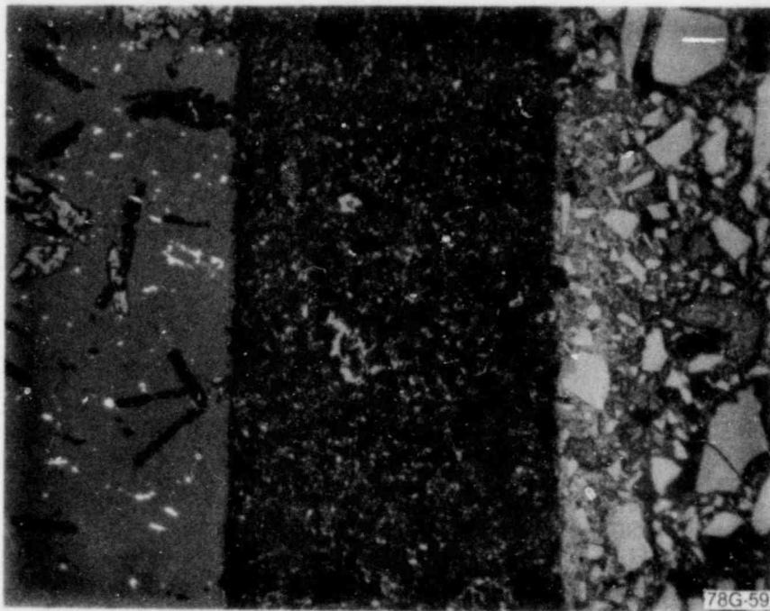
Figure F-7. Interface of ceramic disc, Ceramabond 503, and Sauereisen No. 8 after irradiation (200X).
