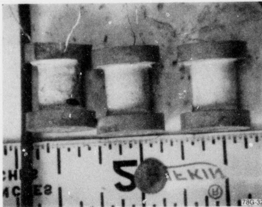
Figure G-6. Irradiated coils prepared on ceramic forms using platinum wire and Ceramabond 503 cement.
