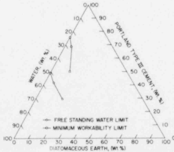
Figure 6. Compositional phase diagram for the solidification of aqueous waste containing 25 wt. % or less diatomaceous earth with portland type III cement (three day cure).
