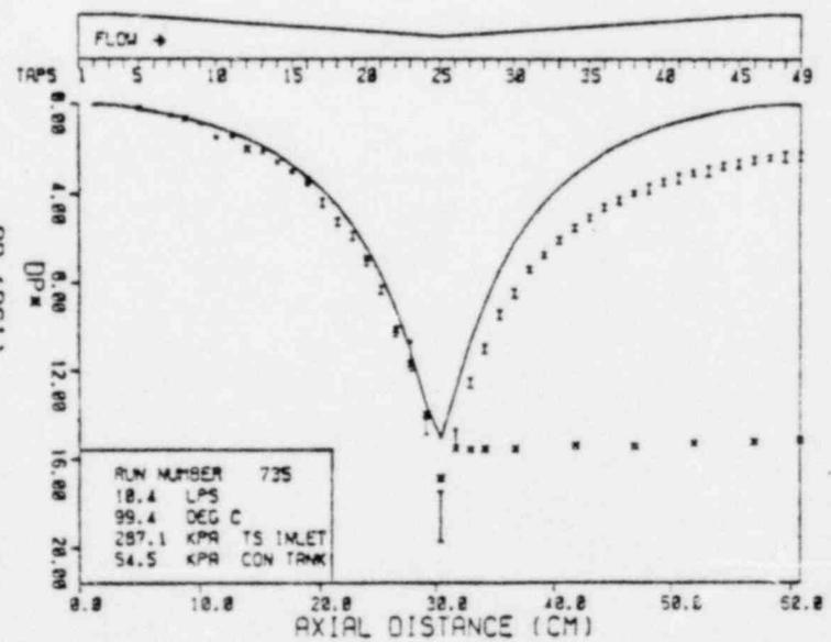
**BML FLASHING FLOWS EXPERIMENT
