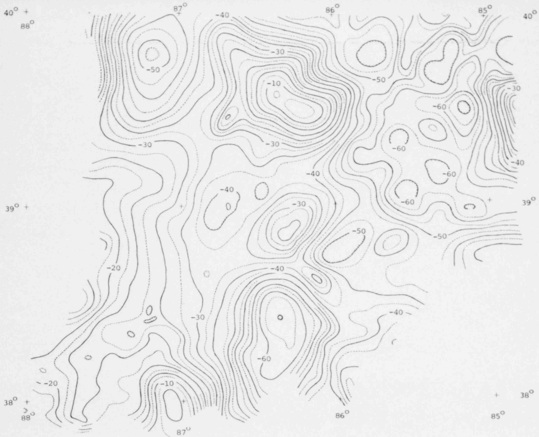
Figure 1. Bouguer gravity anomaly map of southern Indiana-1980. Contour interval is 2.5 mgals. Reduction based on I.G.S.N. 1971, G.R.S. 1967 and a density of 2.67 gm/cc.
