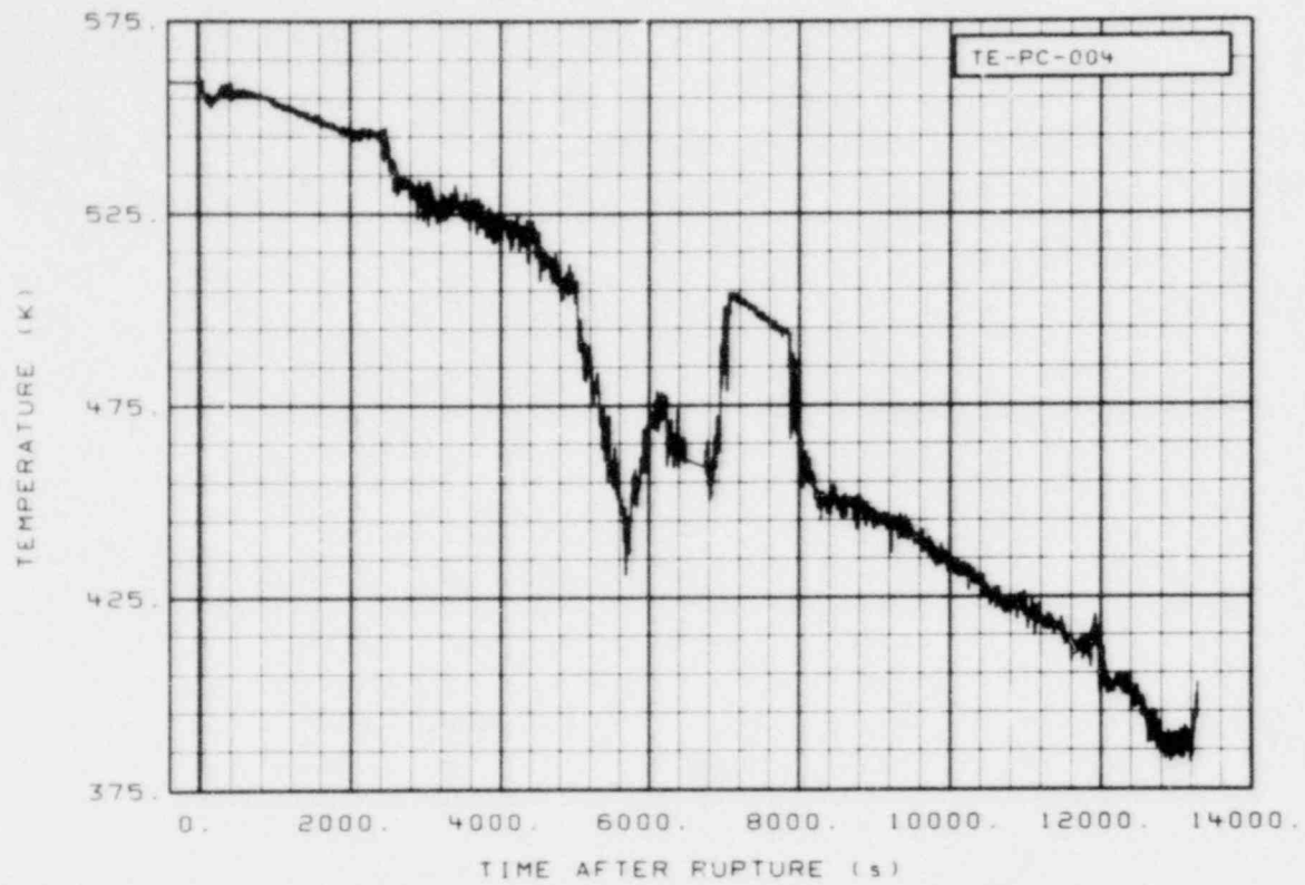
Figure 146. Coolant temperature in intact loop cold leg at bottom of ECC Rake 1 (TE-PC-004) (Qualified).
