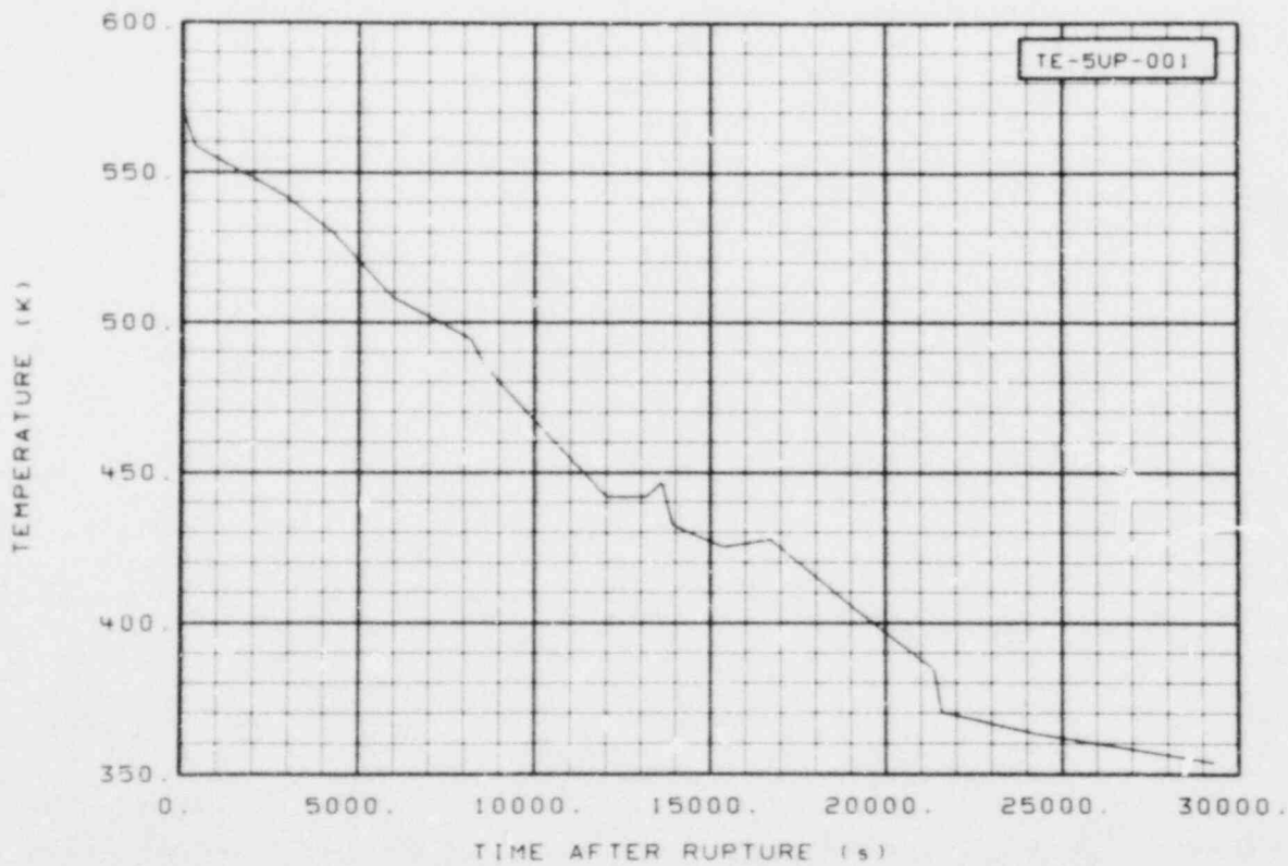
Figure 216. Coolant temperature in reactor vessel at upper end box of Fuel Assembly 5 (TE-5UP-001) (Qualified, uncertainty: \pm 25 K and \pm 300 s).
