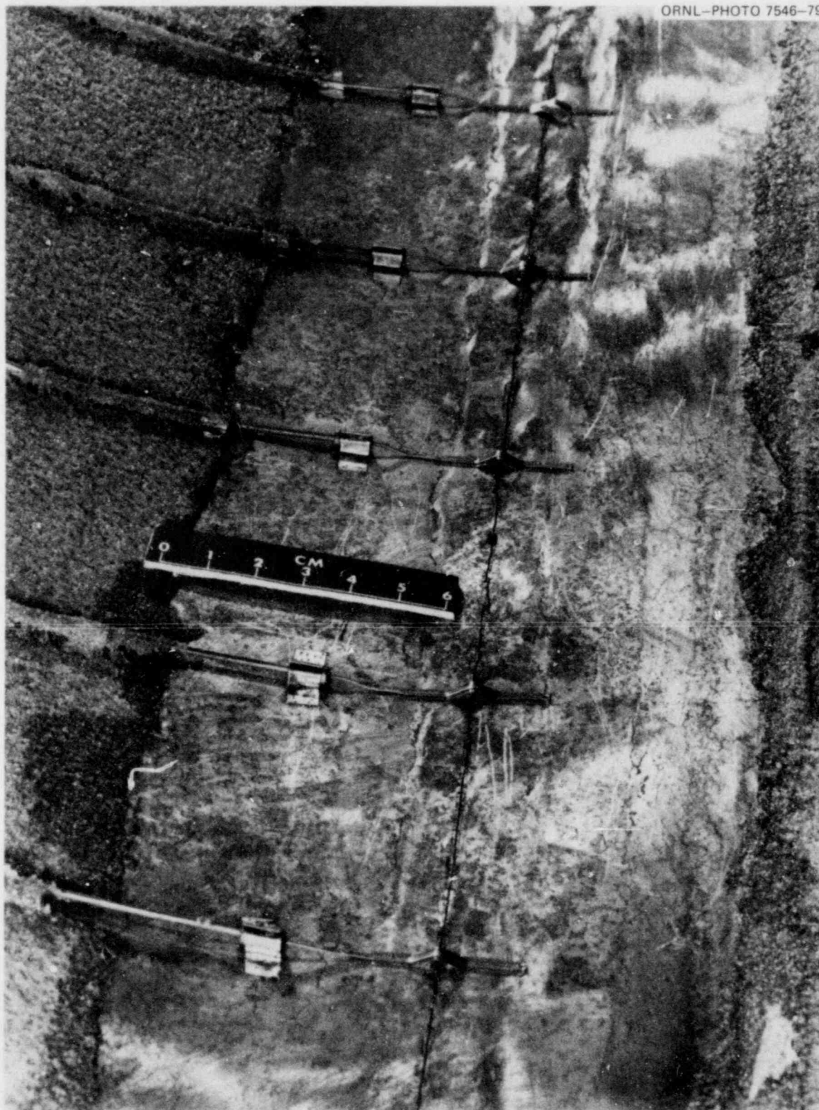
Fig. 6.4. Close-up view of flaw and COD gages in TSC-1 following TSE-5.
