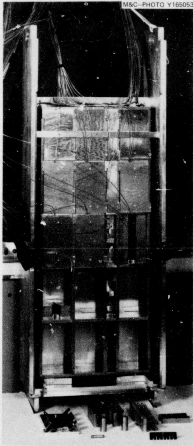
Fig. 4.5. Assembly of capsule for fourth HSST irradiation series.
