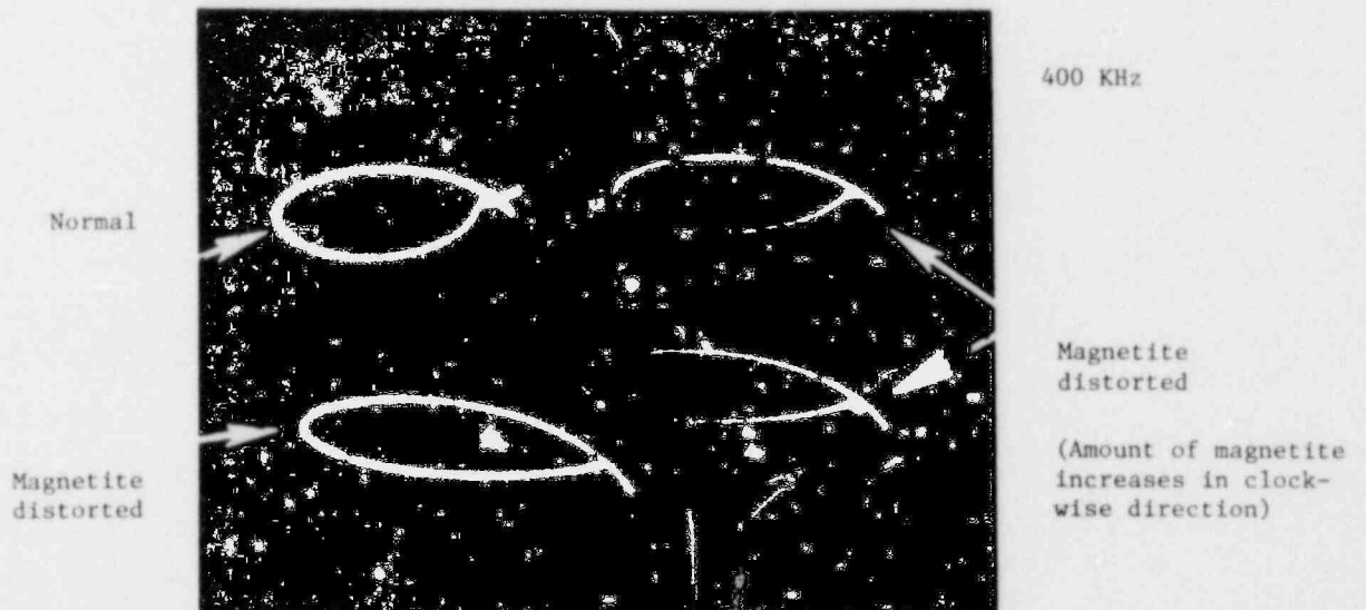
(b) Normal and distorted tube sheet signals
