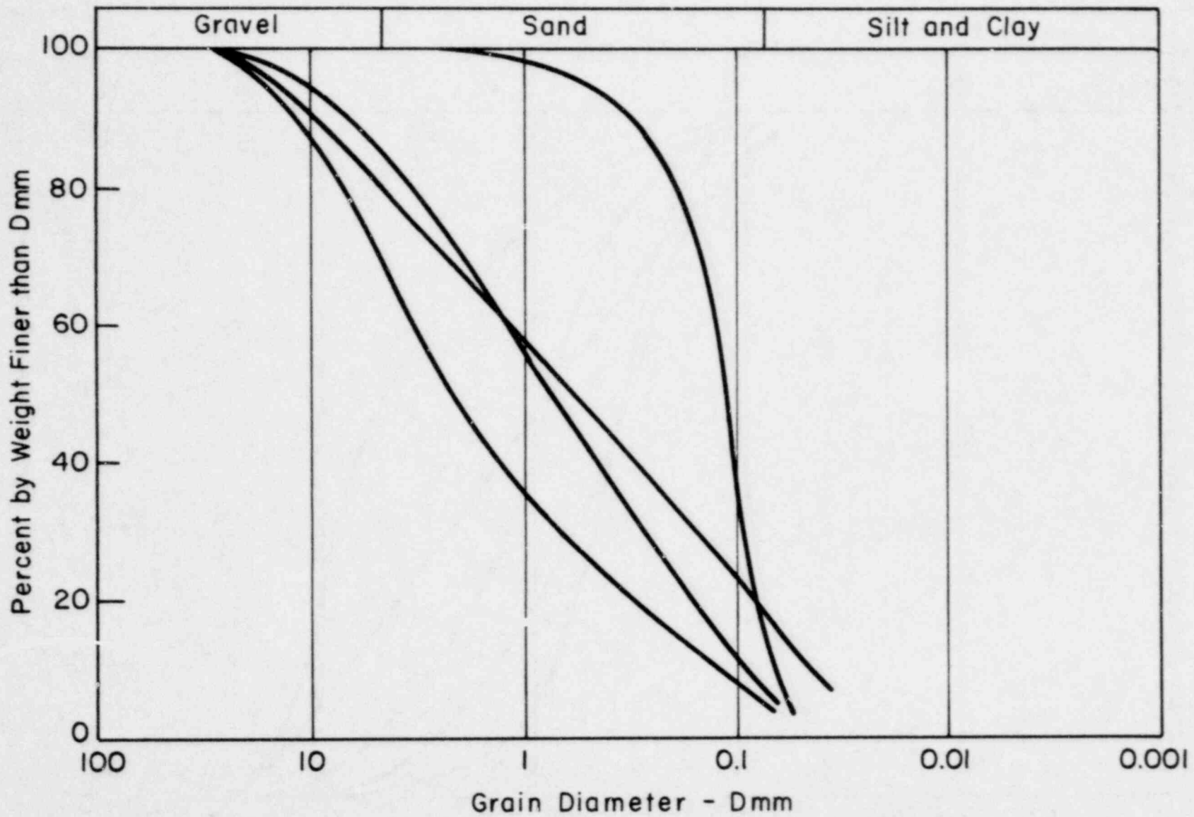
FIG. 14 GRAIN SIZE DISTRIBUTION CURVES FOR SAMPLES OF SAND REPRESENTATIVE OF LIQUEFIED MATERIAL
