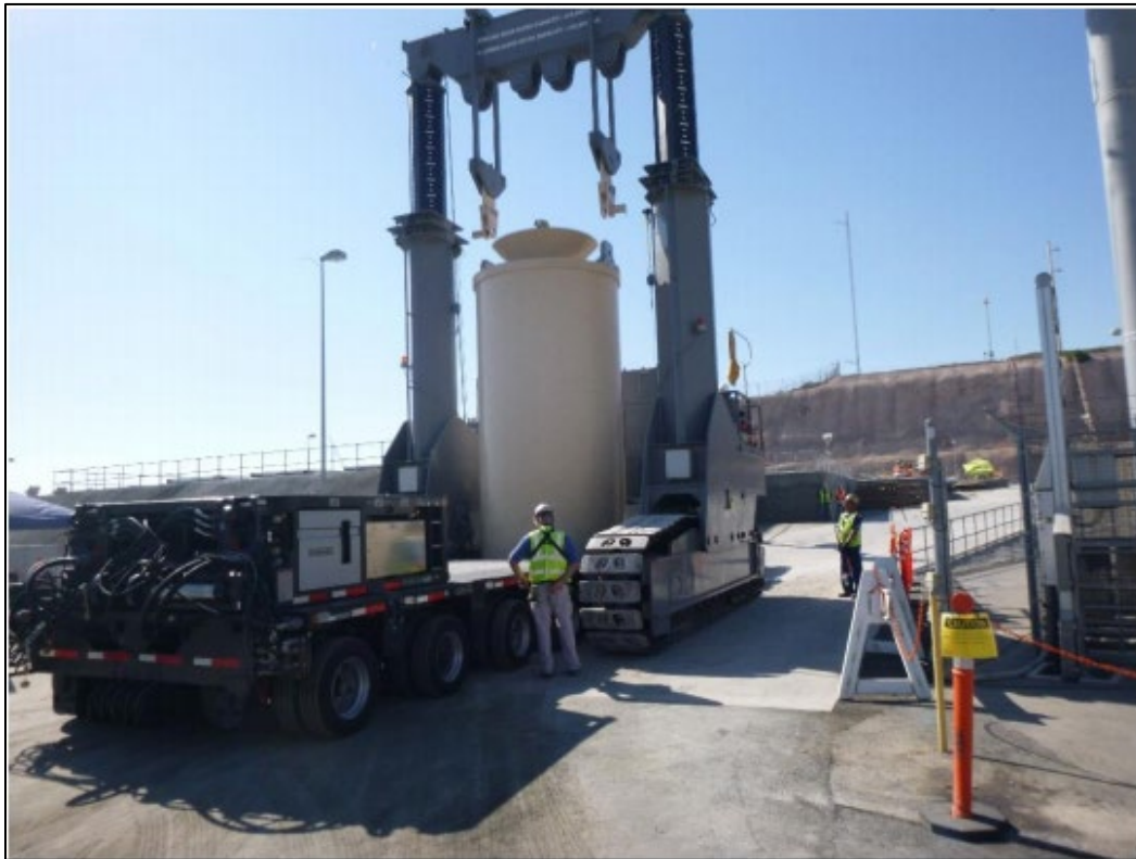
Figure 5. Vertical Cask Transporter during downloading and alignment of a canister.
