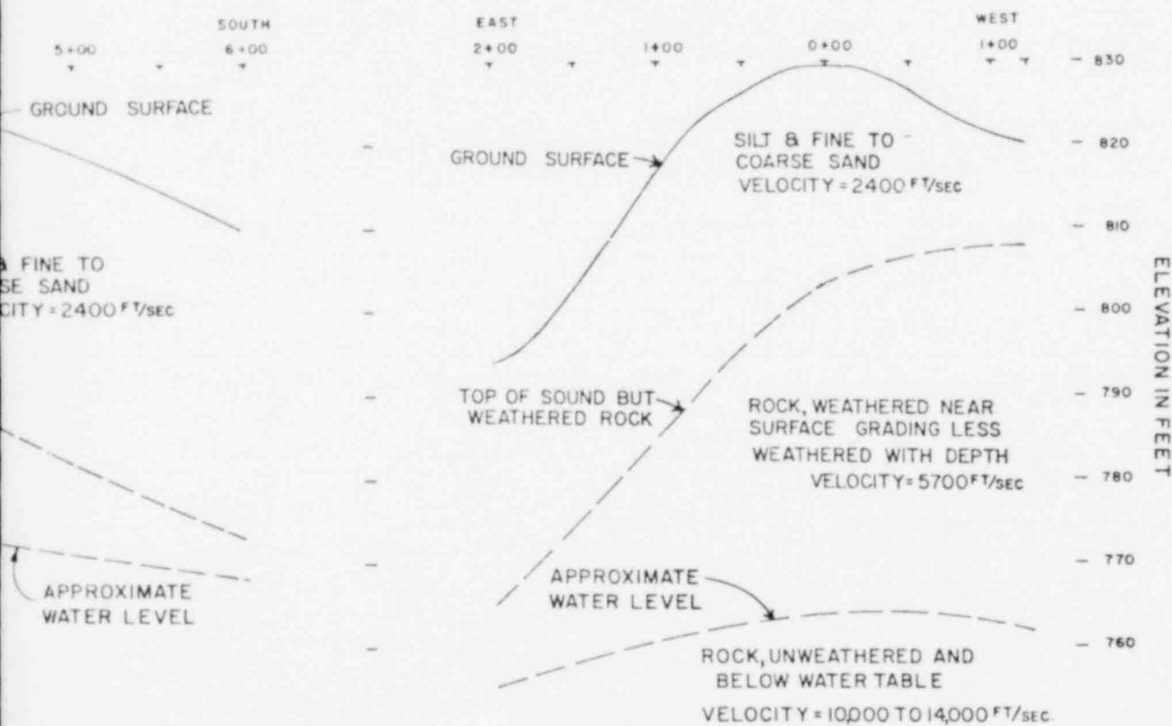
SECTIONS THROUGH SEISMIC LINES
