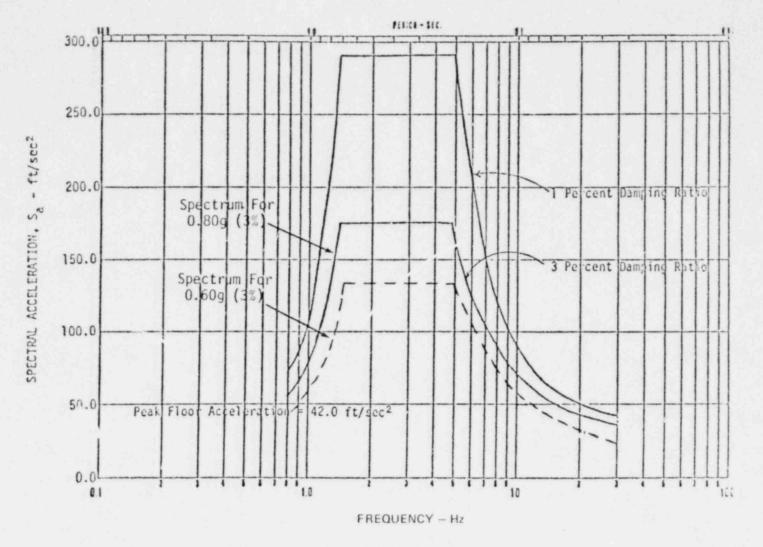
FIGURE 1. ENVELOPE FLOOR RESPONSE SPECTRA FOR HORIZONTAL MOTION AT ELEVATION 611.0 FT 7.0 IN.
