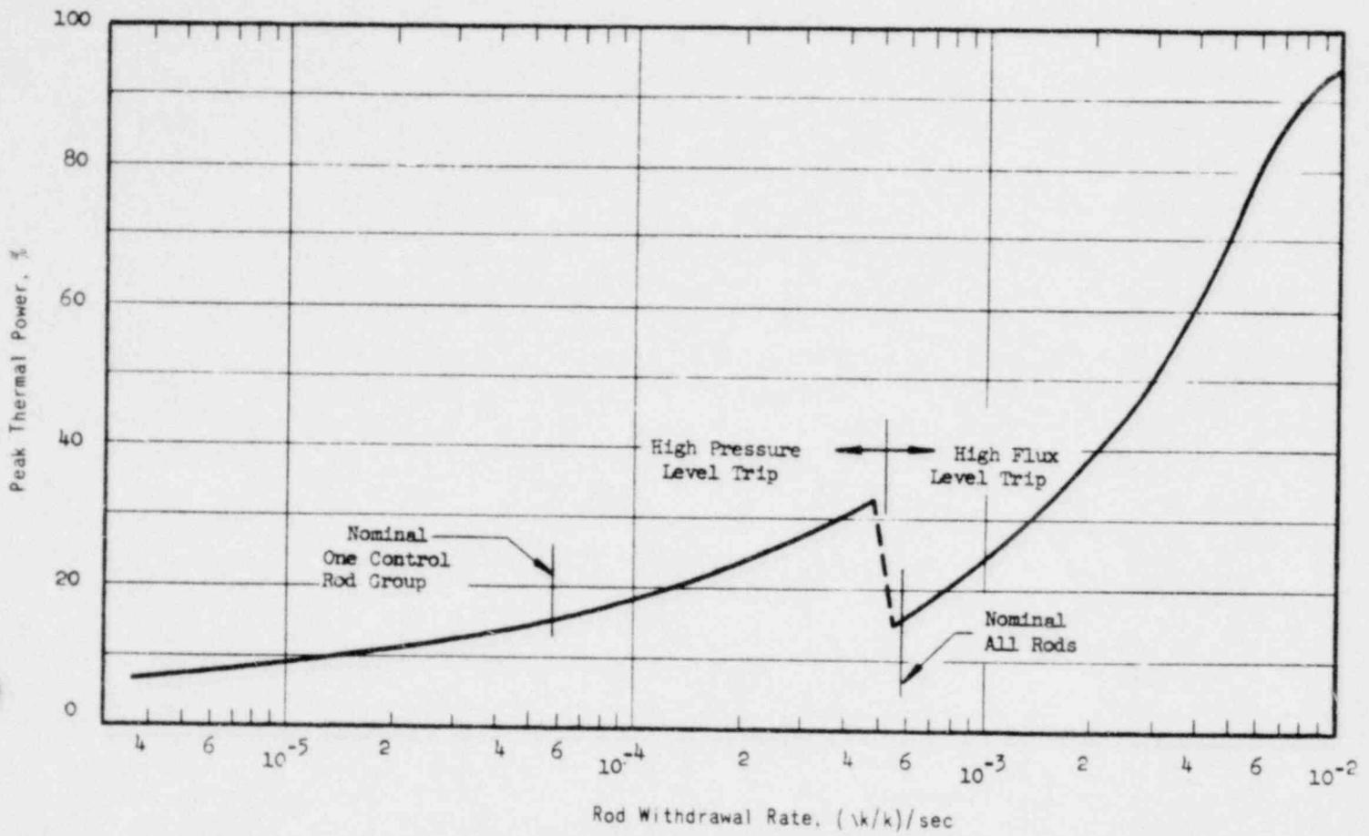
PEAK THERMAL POWER VERSUS ROD WITHDRAWAL RATE FOR A START-UP ACCIDENT FROM 10<sup>-9</sup> RATED POWER
