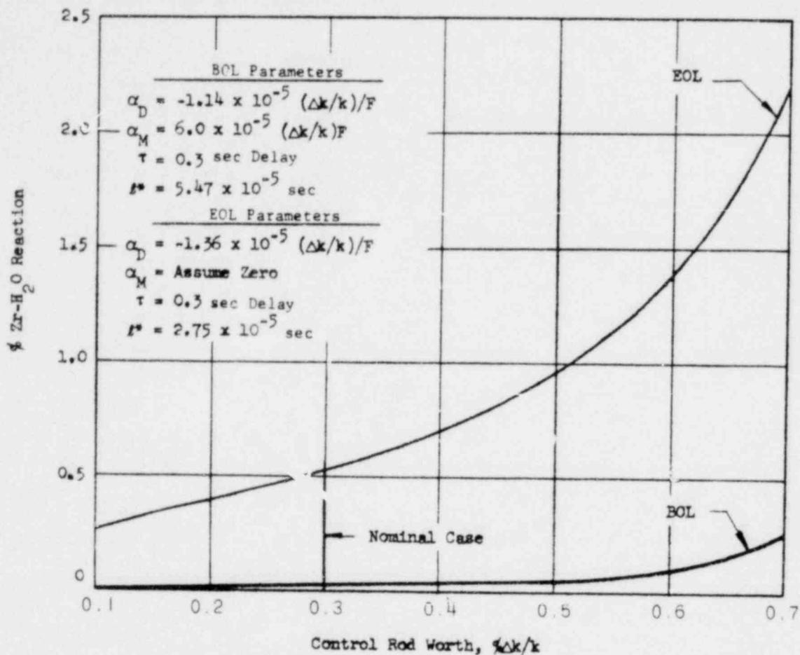
ZR-H<sub>2</sub>O REACTION AS A FUNCTION OF EJECTED CONTROL ROD WORTH AT ULTIMATE POWER
