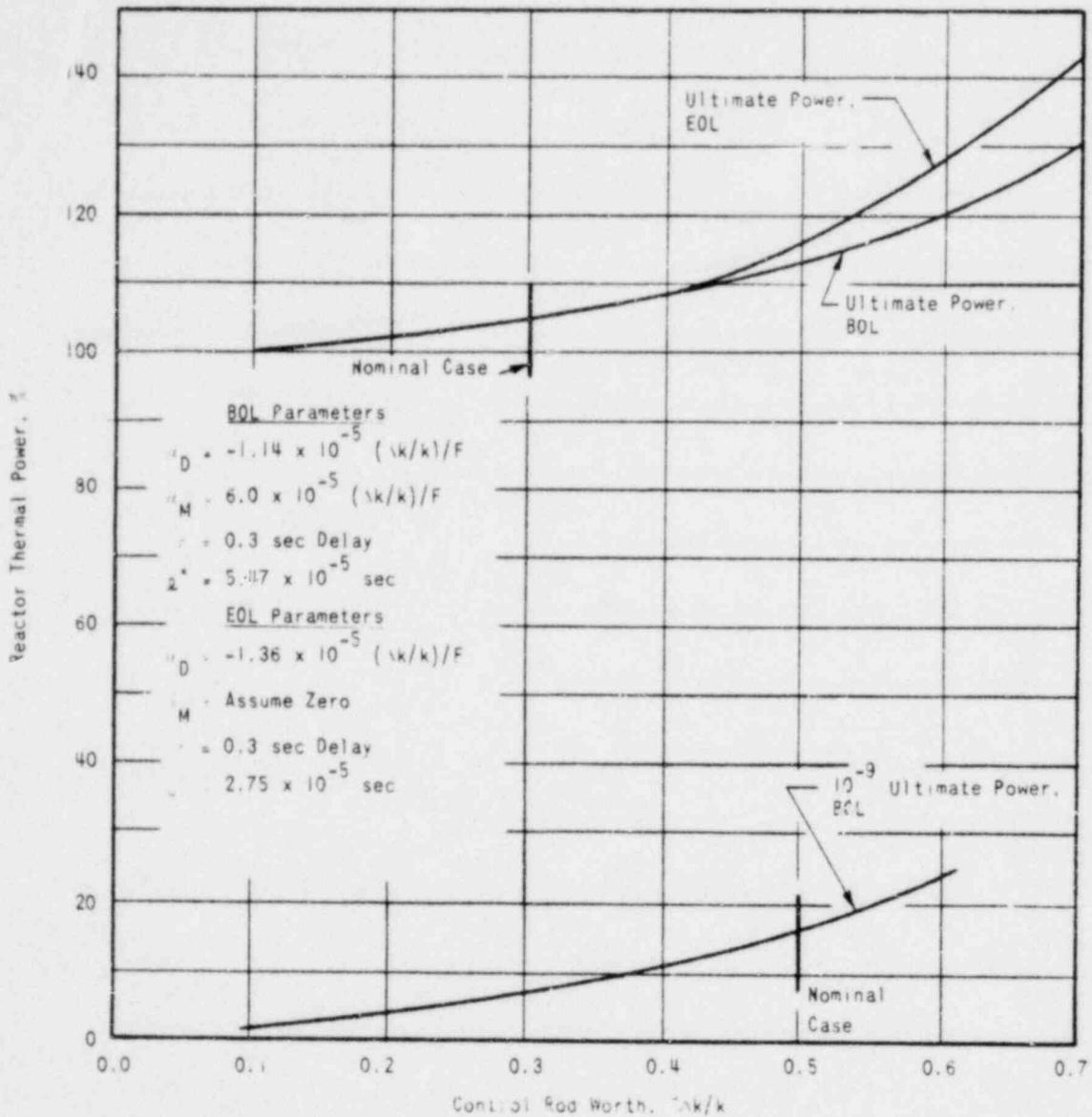
REACTOR THERMAL POWER AS A FUNCTION OF EJECTED CONTROL ROD WORTH
