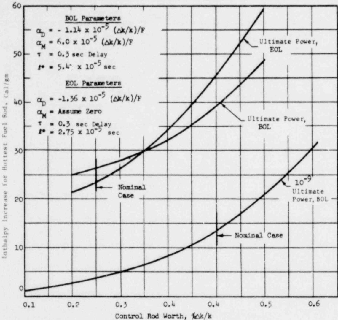
ENTHALPY INCREASE TO THE HOTTEST FUEL ROD VERSUS EJECTED CONTROL ROD WORTH
