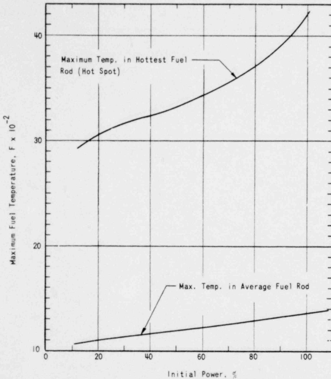
PEAK FUEL TEMPERATURE IN AVERAGE ROD AND HOT SPOT FOR AN ALL-ROD WITHDRAWAL ACCIDENT FROM VARIOUS INITIAL POWER LEVELS
