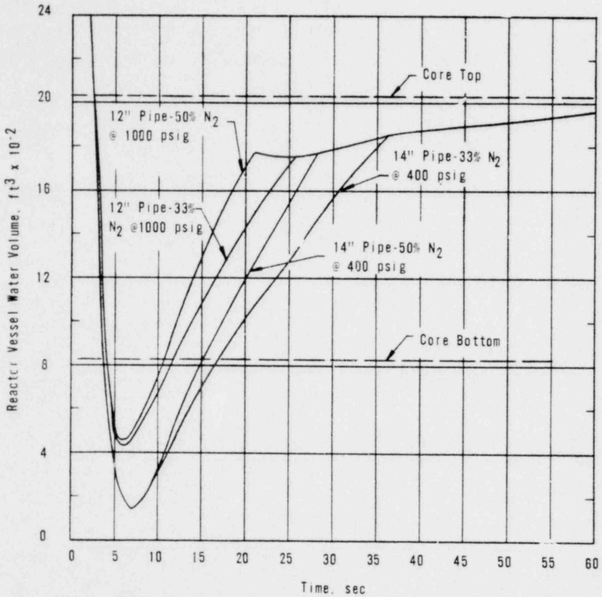
REACTOR VESSEL WATER VOLUME VERSUS TIME FOR
