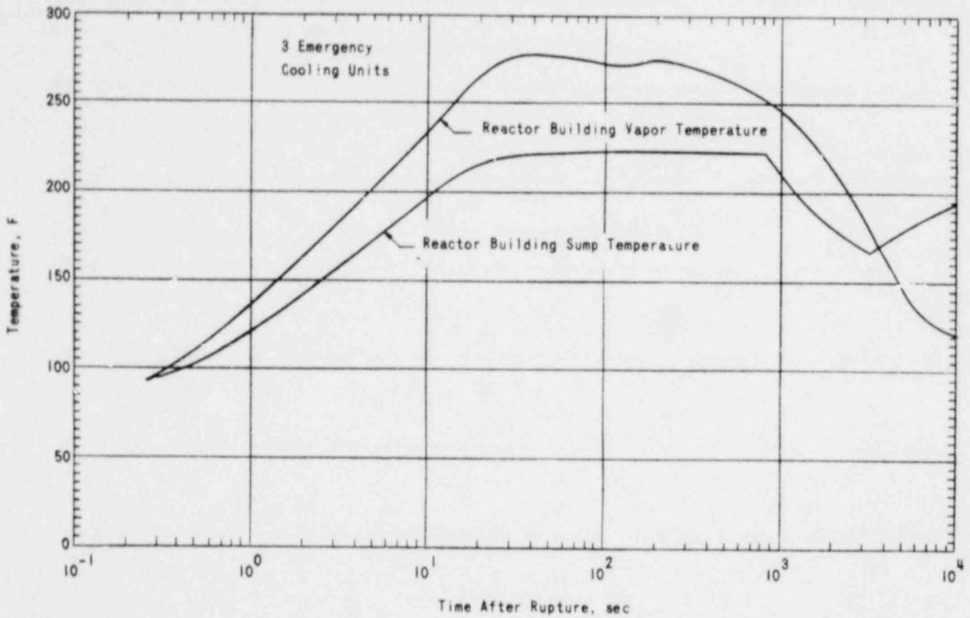
REACTOR BUILDING VAPOR AND SUMP TEMPERATURES
