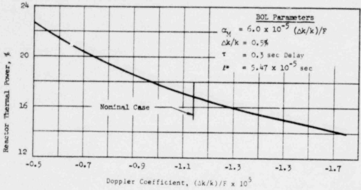
THE EFFECT ON REACTOR THERMAL POWER OF VARYING THE DOPPLER COEFFICIENT ROD EJECTION AT  $10^{-9}$  ULTIMATE POWER
