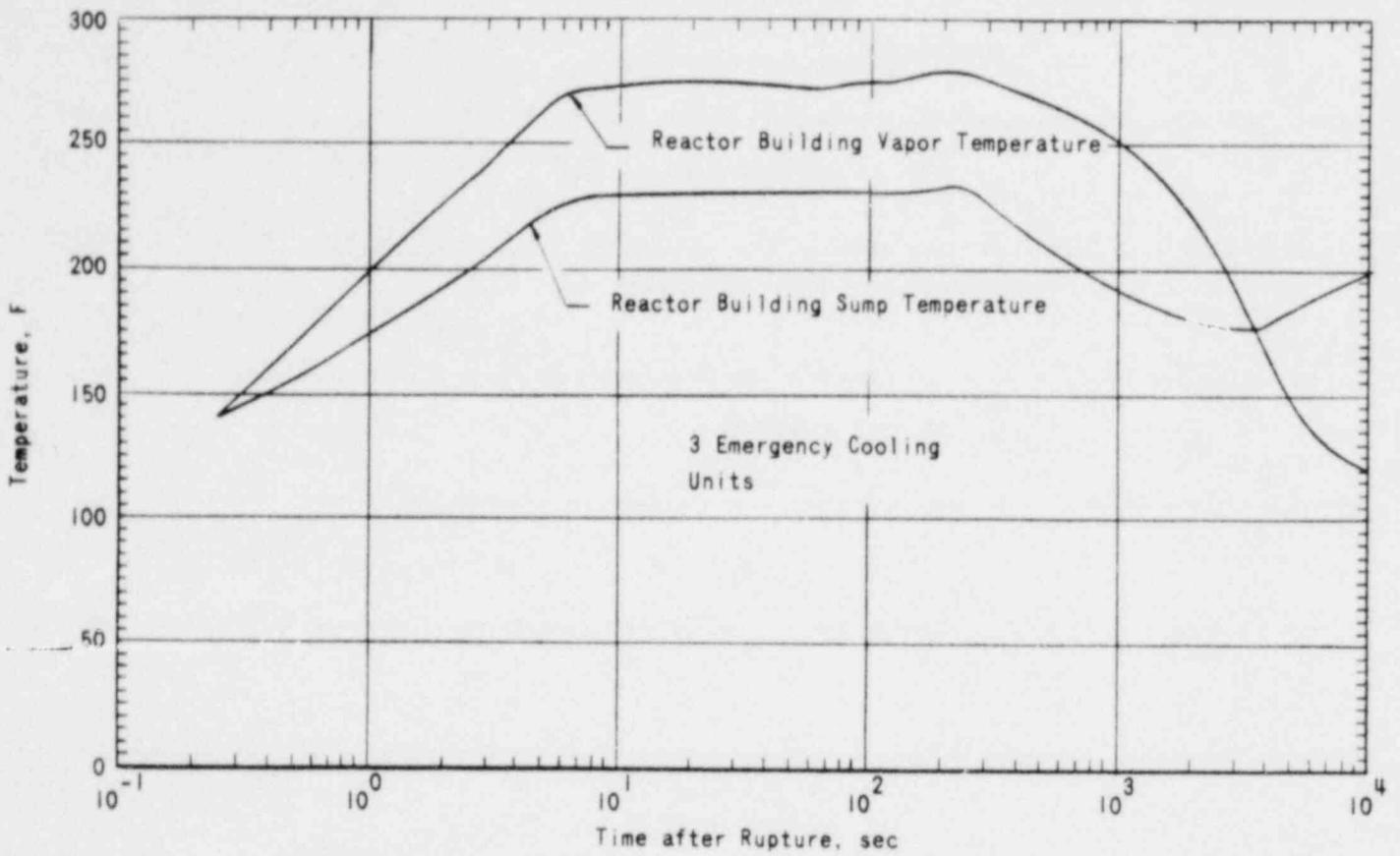
REACTOR BUILDING VAPOR AND SUMP TEMPERATURES
