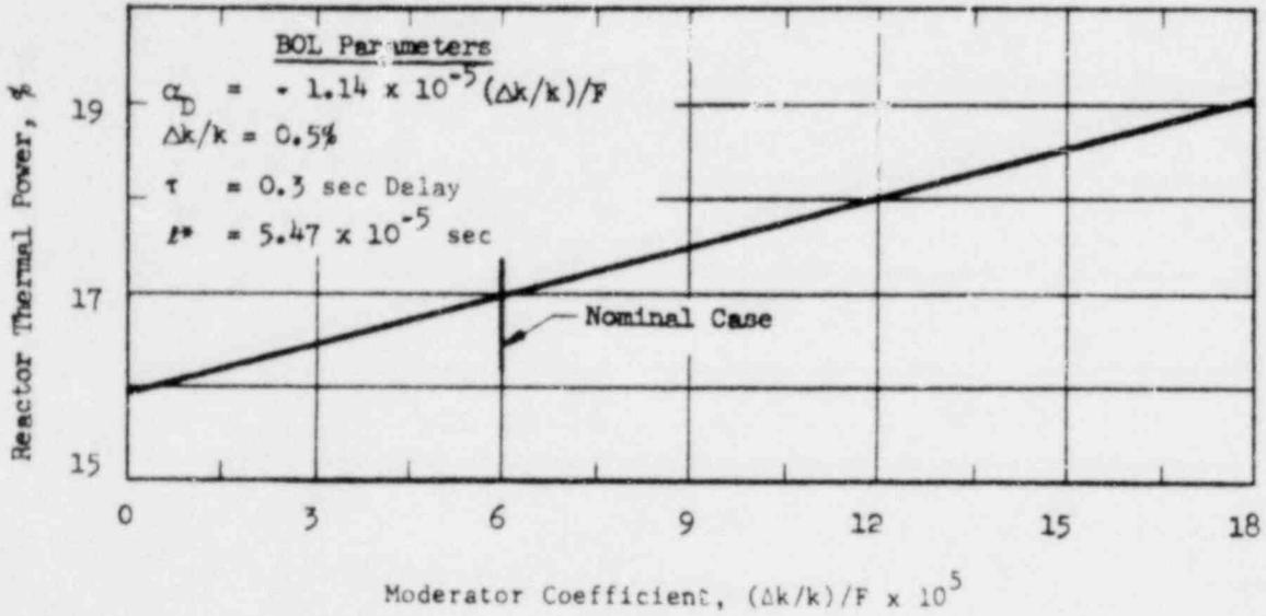
THE EFFECT ON REACTOR THERMAL POWER OF
