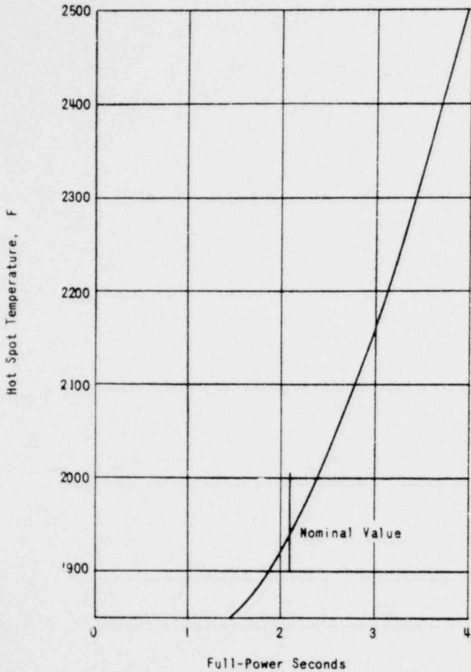
HOT SPOT CLAD TEMPERATURE AS A FUNCTION OF FULL-POWER SECONDS RESULTING FROM VOID SHUTDOWN FOR A 36 IN. ID, DOUBLE-ENDED, HOT LEG PIPE RUPTURE
