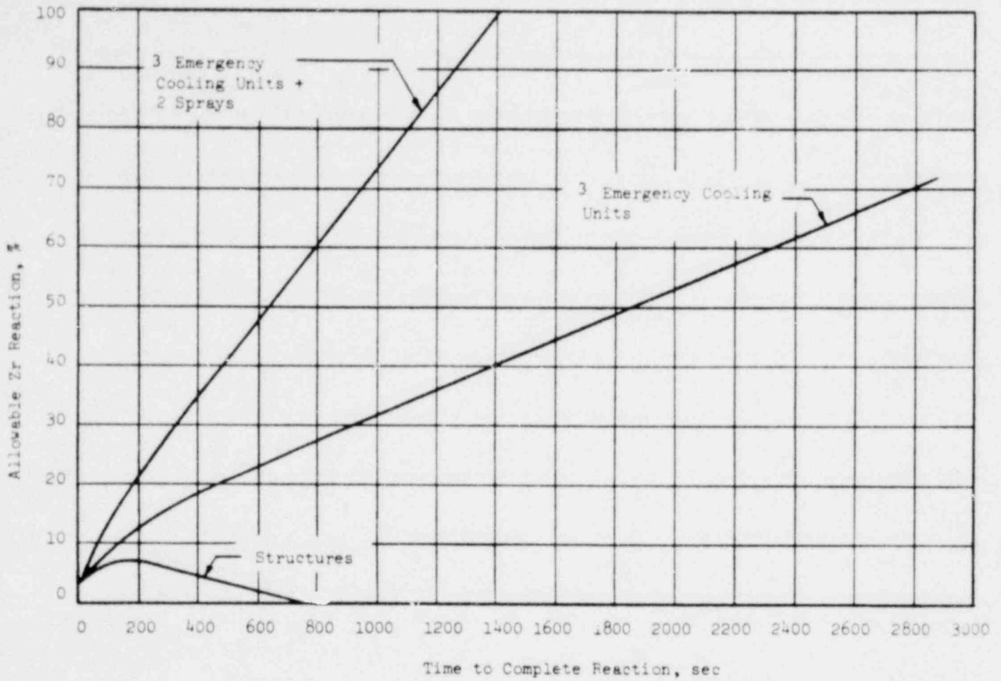
REACTOR BUILDING ZR REACTION CAPABILITY
