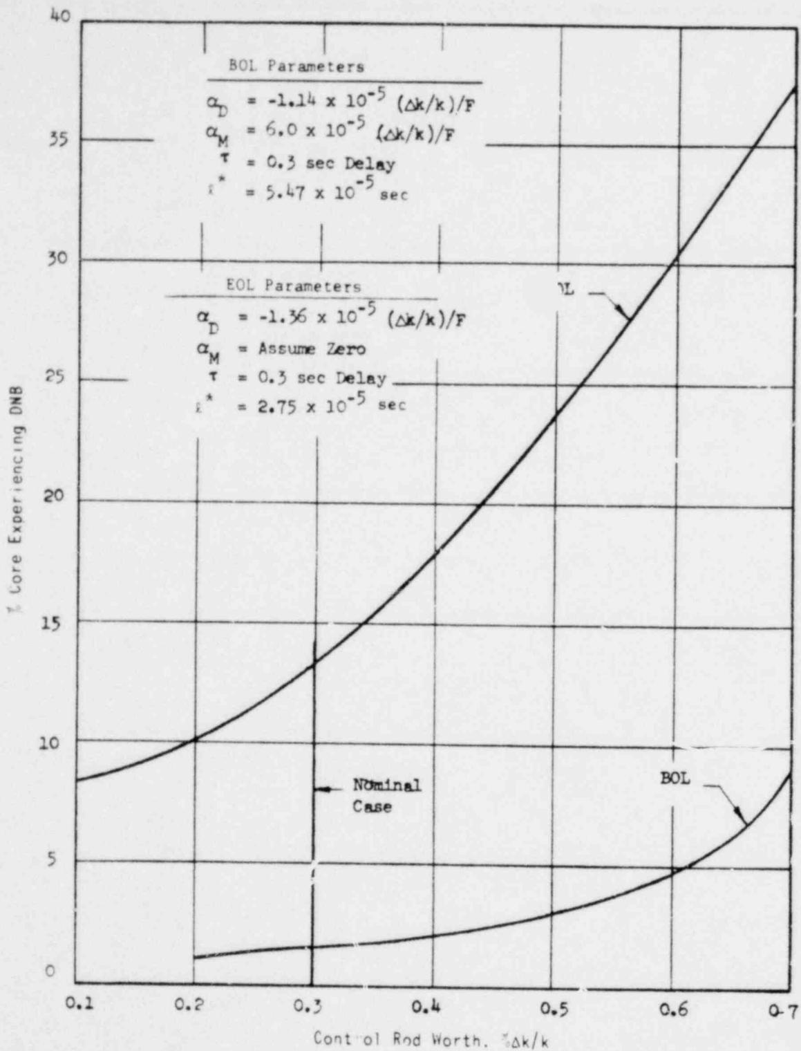
PERCENT CORE EXPERIENCING DNB AS A FUNCTION OF EJECTED CONTROL ROD WORTH AT ULTIMATE POWER
