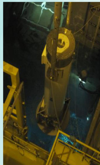
Lifting operation for irradiated materials transport cask
