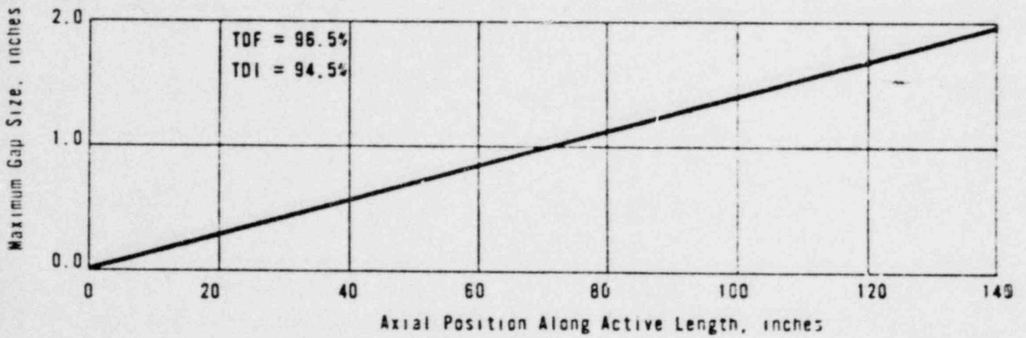
Figure 3-2. Power Spike Factor Vs Axial Position
