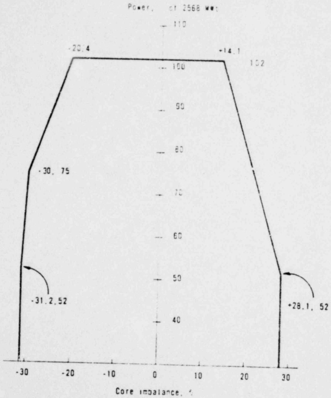
Figure 3-3. Control and Withdrawal Limits for Reactor Power Operation
