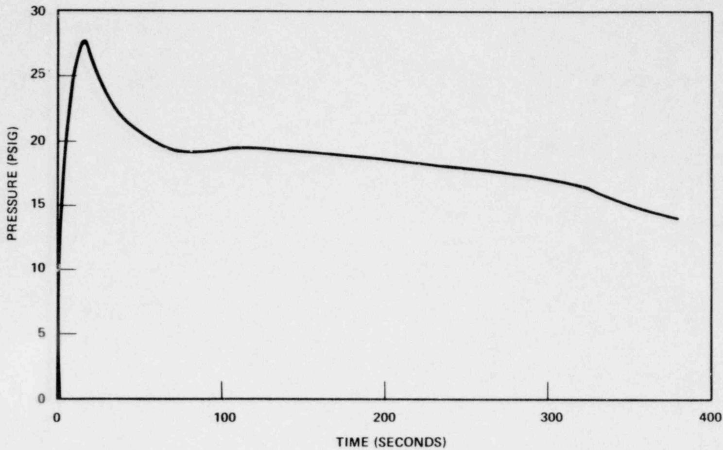
Figure 26 Containment Pressure,  $C_D = 0.6$  DECLG, Pumps Trip
