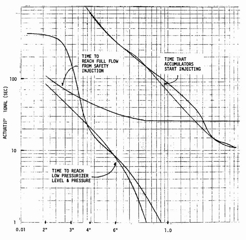
SAFETY INJECTION ACTUATION SIGNAL VS BREAK AREA
