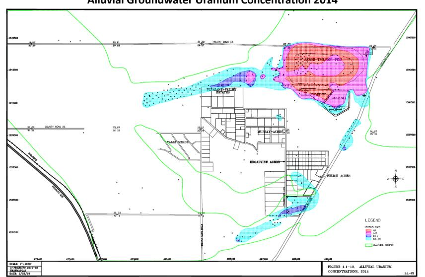
**Alluvial Groundwater Uranium Concentration 2014**
