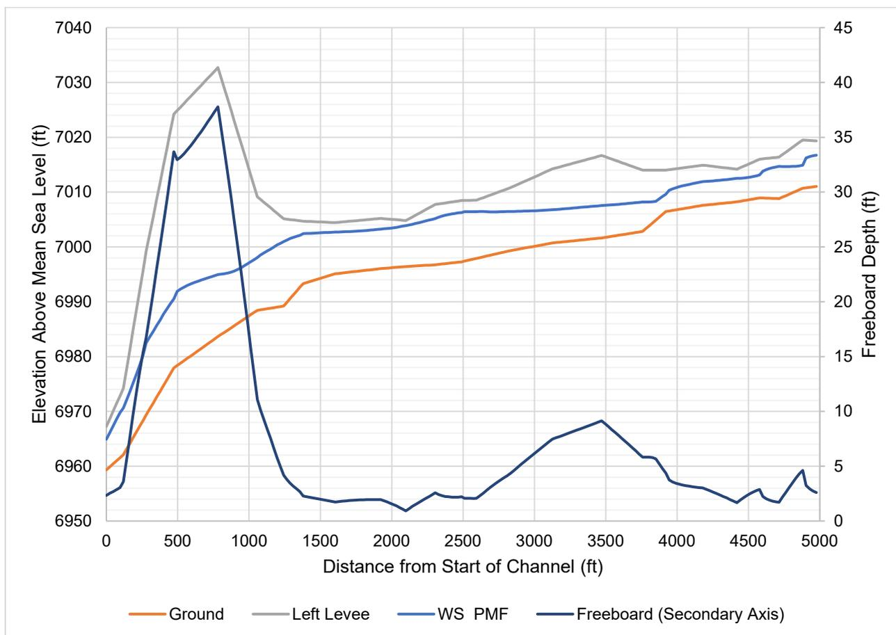
**Figure 5: Plot of North Diversion Channel Water Surface Profile at Maximum Roughness**
