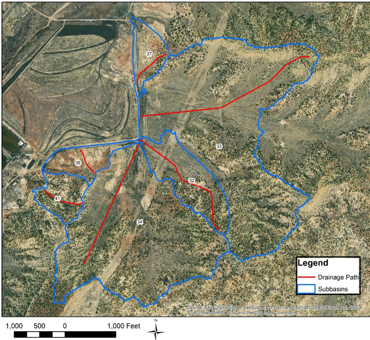
**Figure 1: Contributing Subbasins and Drainage Paths**
