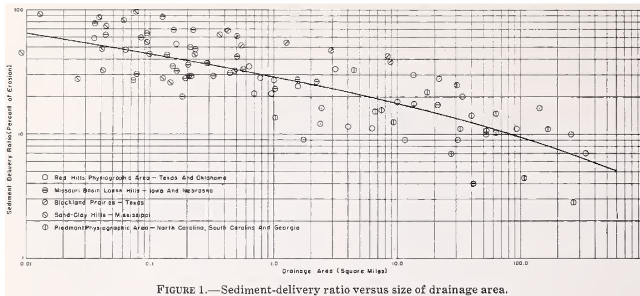
FIGURE 1.—Sediment-delivery ratio versus size of drainage area.
