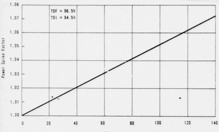
Axial Position Along Active Length, inches Measured from Bottom of Core Figure 3-5 Control Rod Group Withdrawal Limits for Four Pump Operation
